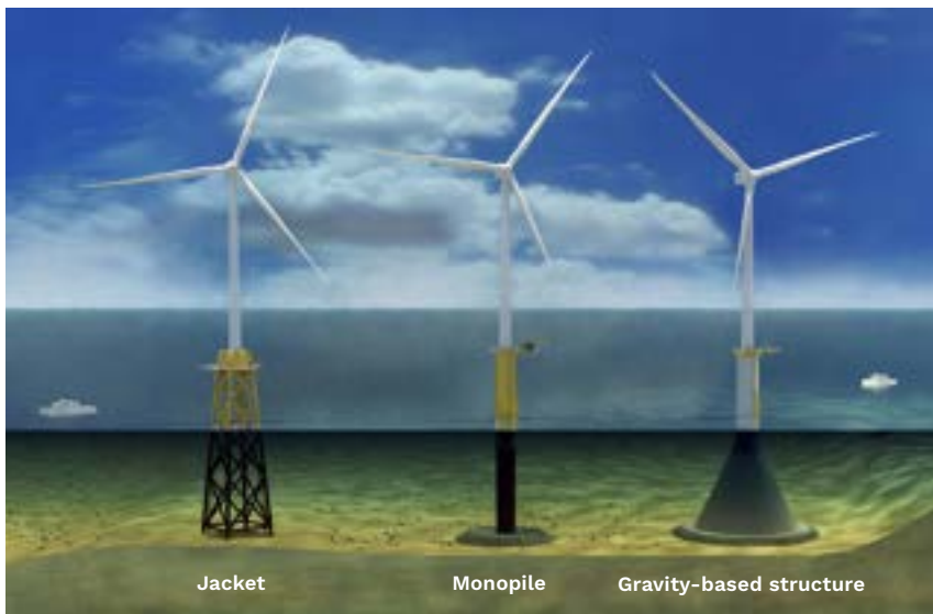
FIGURE 1-6: FOUNDATION CONCEPTS INCLUDING JACKET, MONOPILE, AND GRAVITY-BASED
