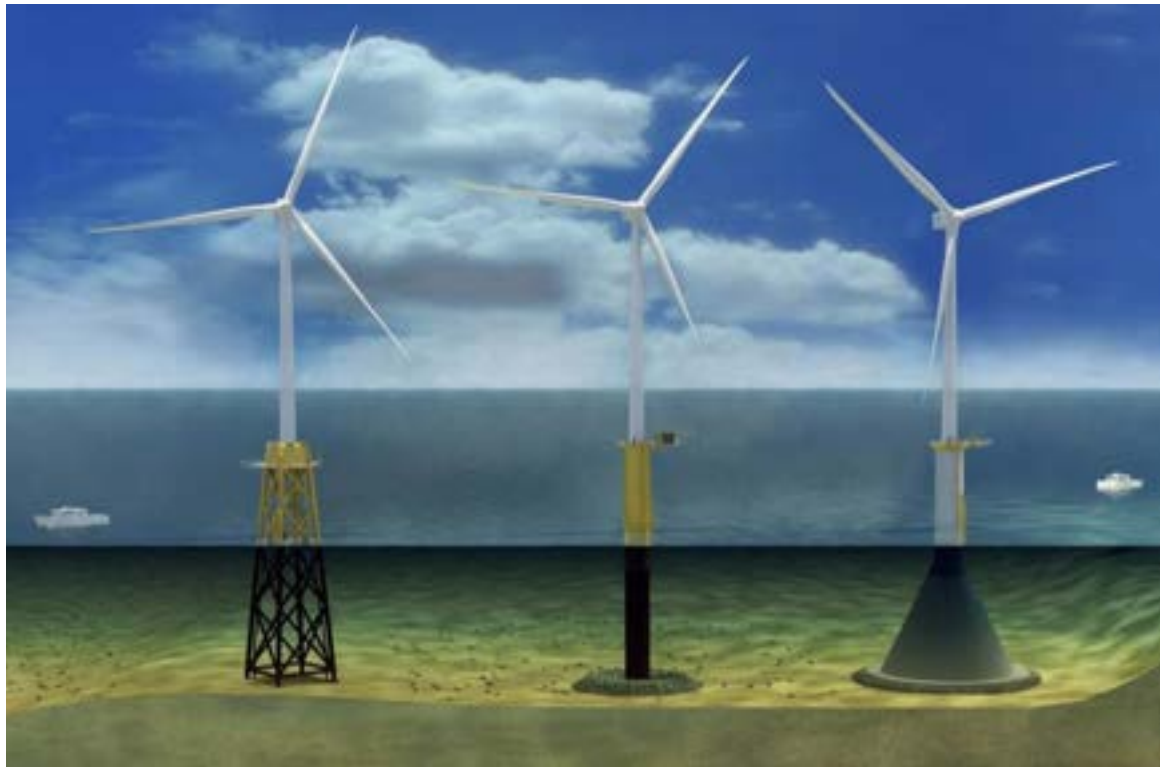
Figure 1: Foundation Concepts Including Jacket, Monopiles, and Gravity-based
