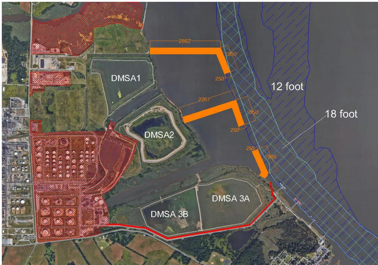
Figure 9: Pier and quay designs for the Delaware site. Shown in orange are three design options based off of the Current Conditions report of three potential sections of the property, referred to from North to South as Oxychem, DMSA2, and DMSA3A as identified in the drawing.
