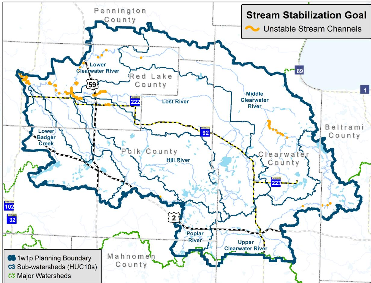
Figure 4.2. Locations for stream stabilization identified by RLWD.
