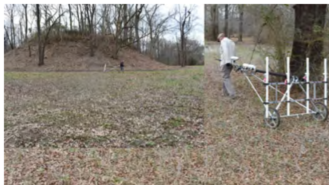
Chet Walker conducts the survey with his Bartington Grad 601-4 fluxgate gradiometer.. Photos courtesy of Christopher Judge.
