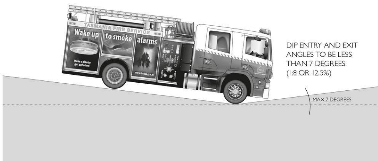
Figure 3 Dip approach and exit angles
