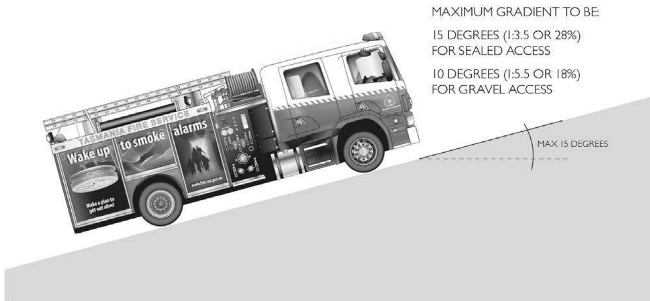
Figure 2 Gradient angles
