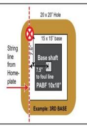
4. Backfill hole around PABF up to field level. Note: Top of Anchor should be 1" below field level. Rubber or Feathered Base Plugs are recommended if Base is not in place.
