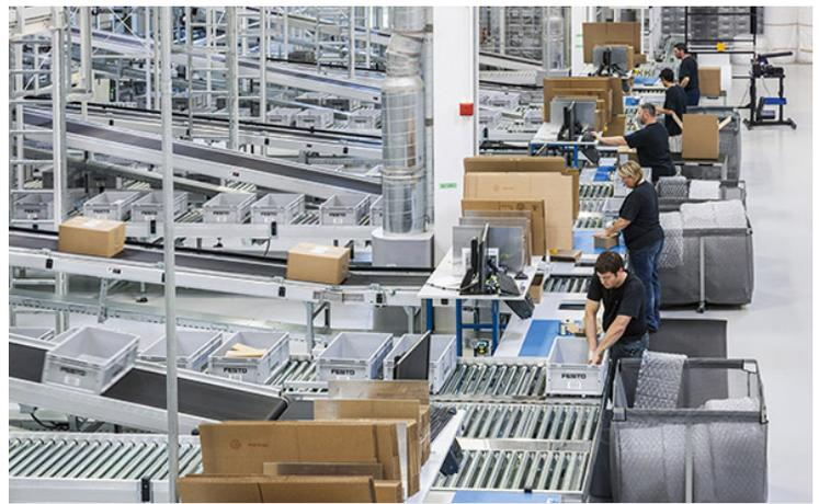
The automated warehouse system enables the processing of large order volumes. With storage capacity of 65,000 bins and the high performance picking and packing stations the system enables Festo to pick and pack more than 1,000 items per hour.
