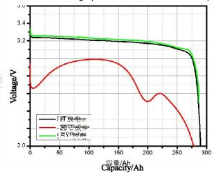
LF280N Discharge performance at different temperatures
