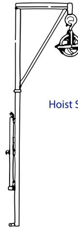
12" diameter for up to 1" rope. 100 lb. capacity.
