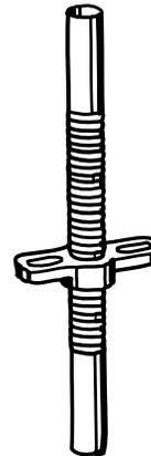
Screw Socket or Screw Jack without Base Plate
