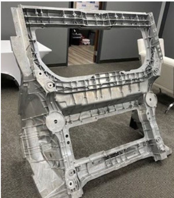
Die Cast EV AL Structural Frame Milling & Drilling Application
