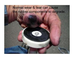
Debris that gets stuck and embedded in the check valve will cause a leak around the debris. Once the debris is removed, an indentation is left in its place, and water leaks through the indentation. Thus, it is most often necessary to rebuild or replace the check valve to stop the leaking. The pictures below show you how debris damages a check valve disc.
