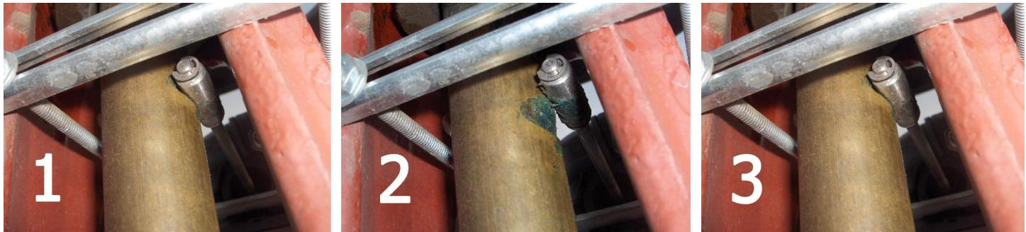
**1:** The arm rests in a groove on the gate valve stem when the gate valve is open.
