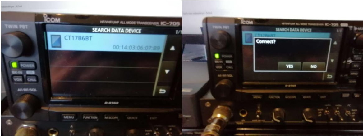
13- You will now get a message saying “Connecting...” (CT17B-6BT in this example)
