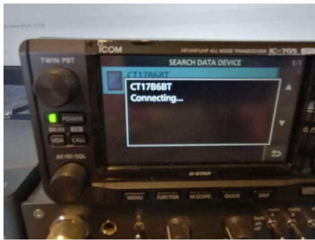
14- Your following message will be to enter the “PIN Code,” hit the OK button, and enter 1234 using the on-screen keyboard (CT17B-6BT in this example)
