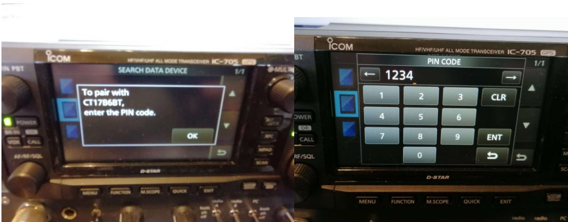
14- Your following message will be to enter the “PIN Code,” hit the OK button, and enter 1234 using the on-screen keyboard (CT17B-6BT in this example)
