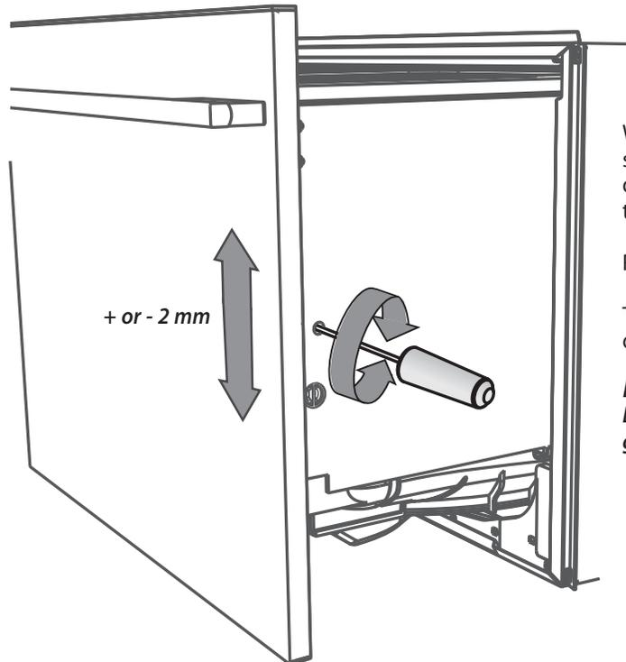
With the front panel fitted, insert an appropriately sized Philips screwdriver into the hole above the door pin and rotate the panel up or down to align the gaps in your cabinetry.
