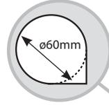
The  $\varnothing 60$  mm services hole should be enlarged to accommodate the extra venting hose by cutting out some material from the bottom corner.
