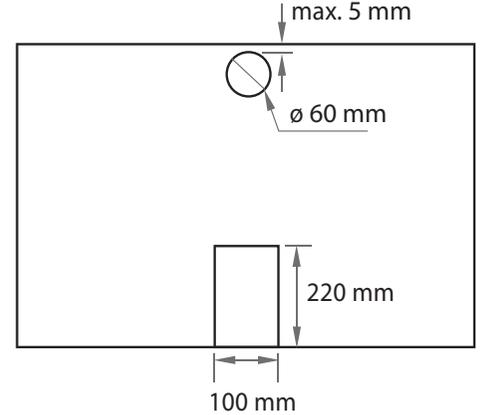
**7c** • INTEGRATED MODELS WITH REMOTE (NZ AU) ONLY - PREPARATION FOR EXTERNAL VENTING THROUGH ADJACENT CABINET
