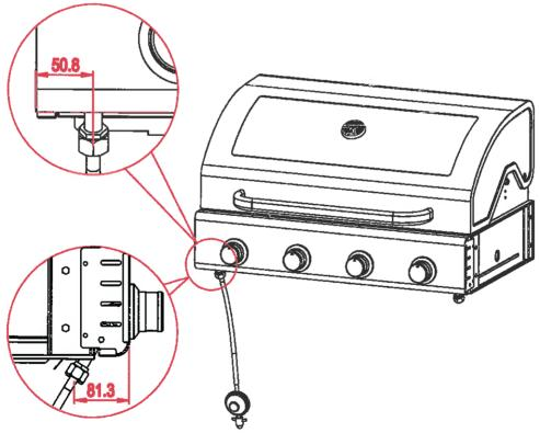
Manifold connection is 1/2" BSP at the front left underside of the BBQ head as shown. Manifold connection is 81.3mm from the front edge of the bbq, and 50.8mm from the left edge of the BBQ
