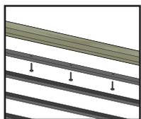
Every rake and level panel is predrilled on the top rung and comes with screws for attachment to the handrail. Screws are also included for the bottom of each panel.
