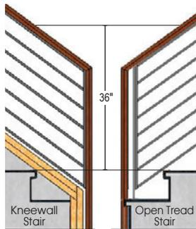
36" Rake rail height and 36", 39" or 43" level run rail heights. Rail heights may vary due to field conditions or preferences
