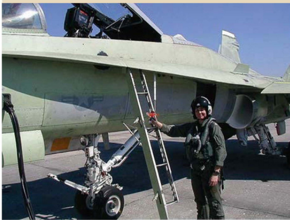
Kim Dyson prepares to fly a functional check flight in an aircraft that has just had its center section replaced. Once an aircraft passes a check flight, maintenance teams will paint over the green primer before releasing the airplane back to its squadron. (Smithsonian American Women's History Museum)
