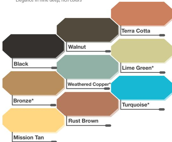
\***Stain-Crete** colors Weathered Copper, Lime Green, Bronze, and Turquoise are for interior applications only. Stain-Crete must be applied on concrete that has cured a minimum of 28 days and is not subject to hydrostatic pressure. Please see technical data sheet for complete information.
