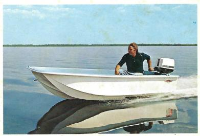
The McKee Craft Pirate is the boating industry's answer to a safe and rugged 10-foot utility boat. Standard features include two fiberglass bench seats, forward and aft towing eyes, stern cleats, bow chocks, and internal conduit in which you may install running lights.
