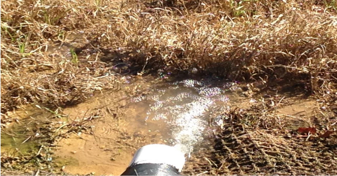
Clear water coming from skimmer discharge pipe at 12:07 p.m. (3 hours after FLOC application)
