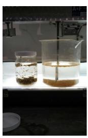
Innovative Equipment Solutions determined that the water from a County Landfill could be treated effectively with FLOC-20G. The sample water was treated with FLOC-20G in the above sample water from the landfill. The suspended solids in the water quickly settled out after the addition of the FLOC-20G and agitation. Treatment pictures are shown above.
