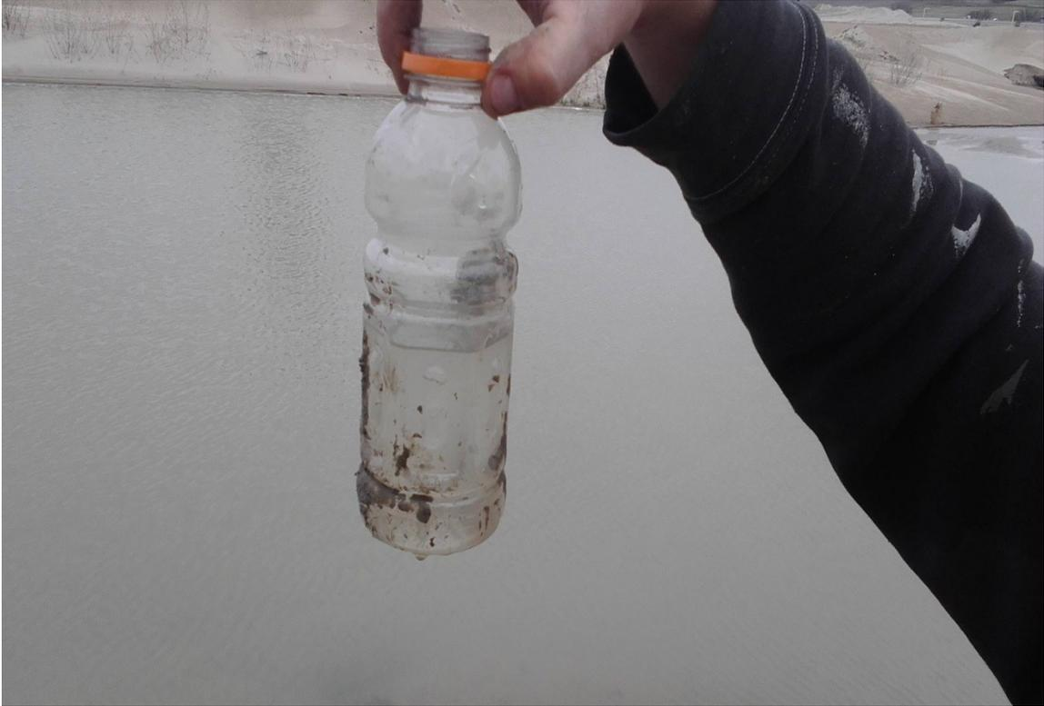
FLOC™ 05 was applied through re-circulation pump at  $\frac{3}{4}$ # per 1,000 gallons.
