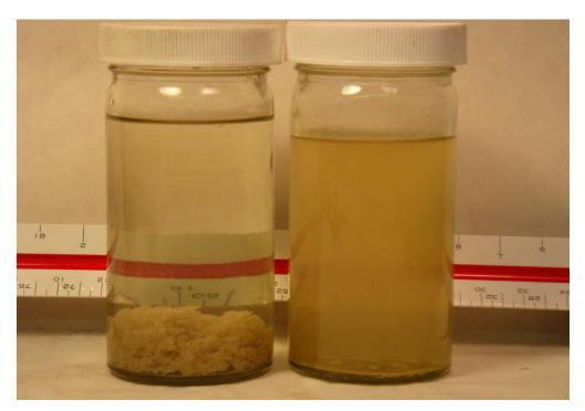
The jars shown above are produce water that has been treated with Floc (left) and untreated (right). The suspended solids decreased from 120 ppm to less than 5 ppm. Floc dosage in further testing was measured to be 0.1 gram/1 grams or 8.34 lbs/1,000 gallons. Traditional pretreatment chemistries are not as effective in contaminants removal.
