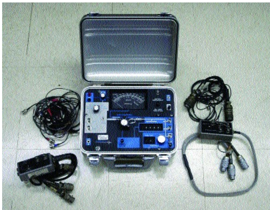
Barfield 2548 test unit with adapter harnesses and test lead package.
