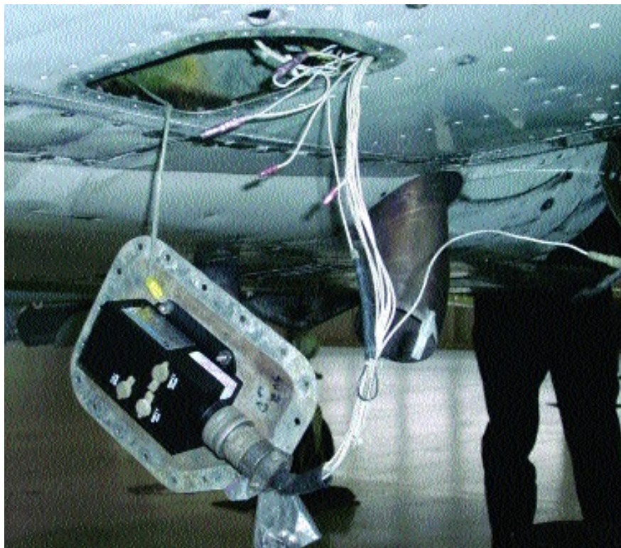
Signal Conditioner, note the adjustments marked on case.
