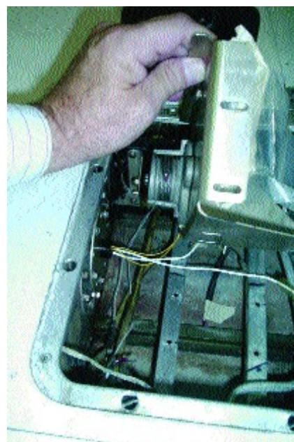
Autopilot servo is held out of the way to show fuel probe stand-off and wiring is in its native element.
