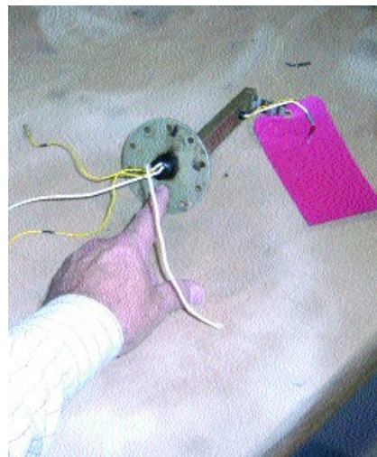
Defective potted feed-through on stand-off assembly.
