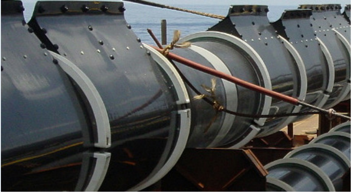
Figure 10: Lankhorst fairings for VIV suppression. Source [53].
