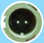
External +24 VDC battery back-up connector. This gives the flexibility of powering the BDA with both an AC and DC source. If both sources are connected, the BDA will automatically select the stronger voltage source for power without ever going offline.
