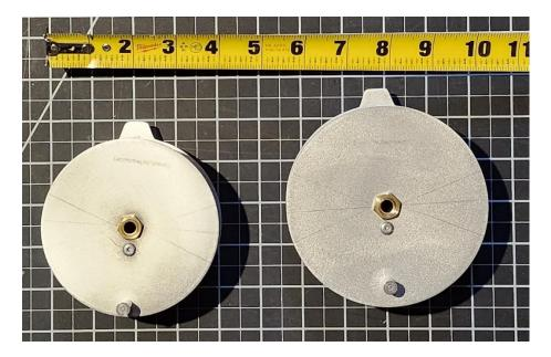
Standard reel size is 4" outside diameter. Large reel is 4.5" diameter. Both sizes have 2" arbor. Made from aluminum. Larger reel holds more/heavier line. 3" reel (not shown) has 1.5" arbor. Reel capacities.
