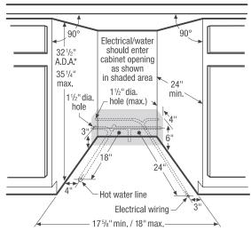
\*A.D.A. installation, (32½") beneath 34"-high countertop may be accomplished by adjusting toekick and leveling legs.
