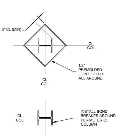
**Typical Isolation Joint Details** SCALE: 3/4" = 1'-0"
