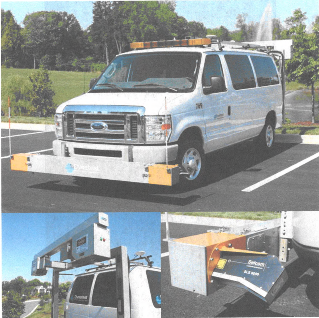
Figure 5 Dynatest PCSS Equipped with LRIS
