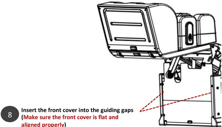
**Fig.6: Footrest Assembly: Chair Front Cover Reset**
