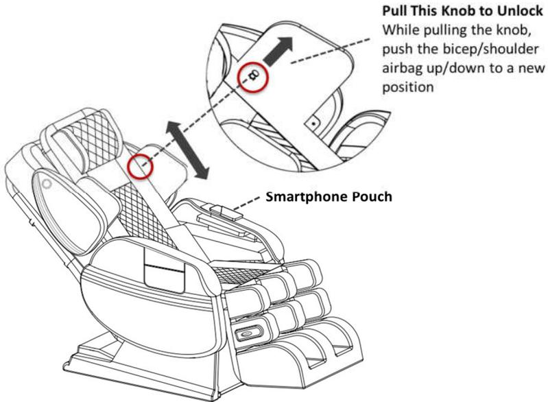
**Fig.21: Bicep/Shoulder Massager Position Adjustment**
