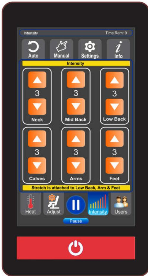
Fig.18: Intensity Adjustments
