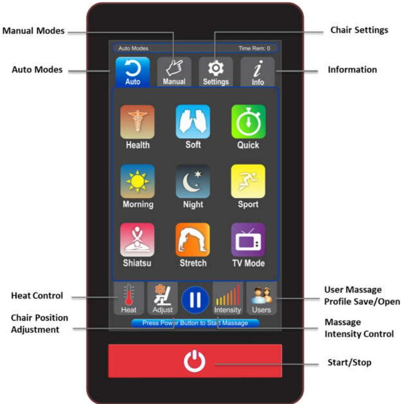
Fig.10: Main Screen and Start/Stop Button
