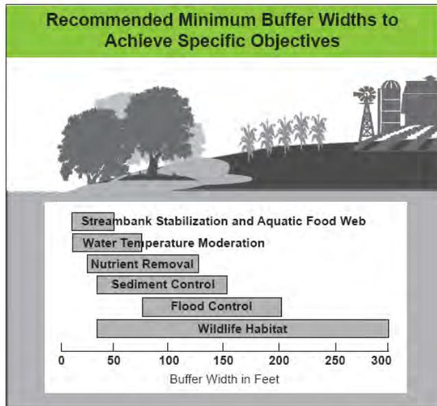
**Figure 5.1 Buffer Widths and Objectives**
