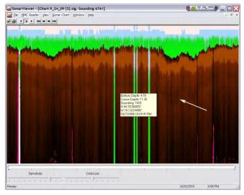
Color-adjusted sonar chart showing secondary return for sediment thickness
