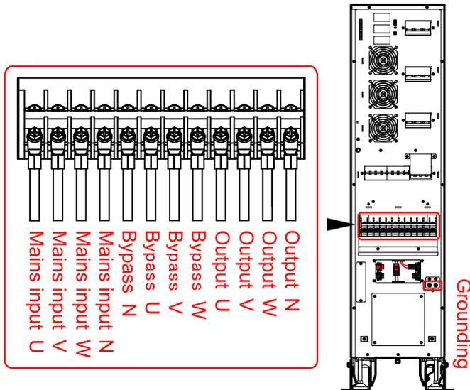
Figure3-21 Wiring diagram of 33 mode
