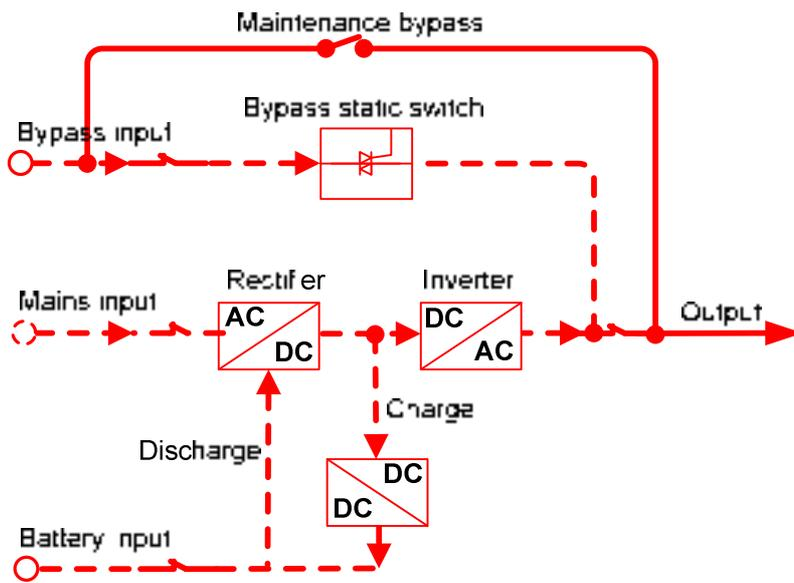
Figure2-16 Maintenance bypass power supply mode (the thick solid line stands for the energy flow direction)
