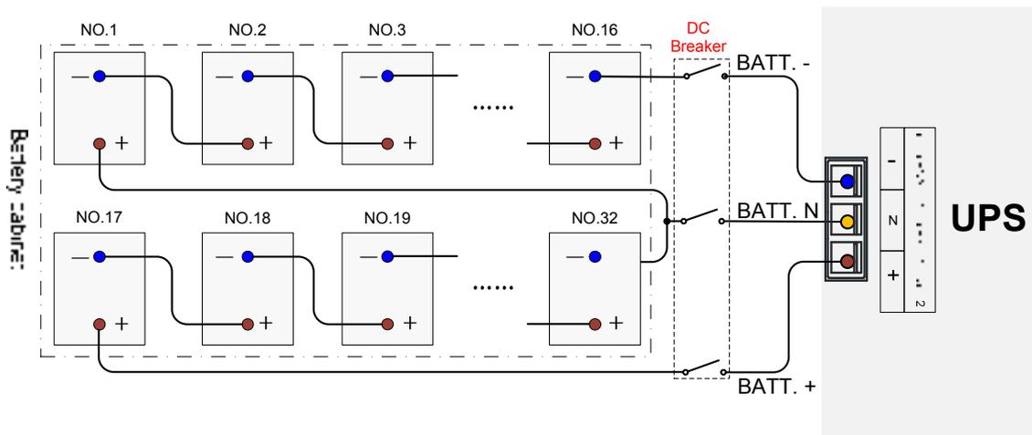
Figure3-25 Wiring diagram 1 of external batteries
