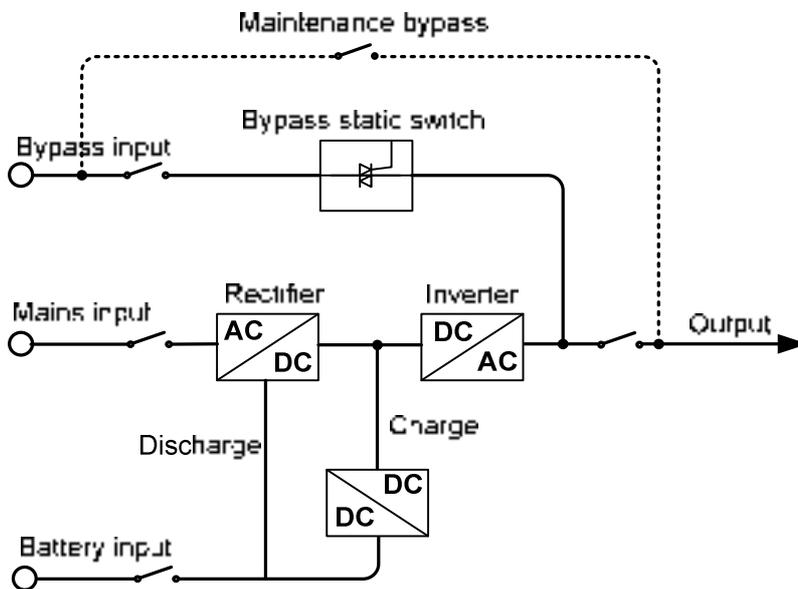
Figure2-12 Work principle diagram
