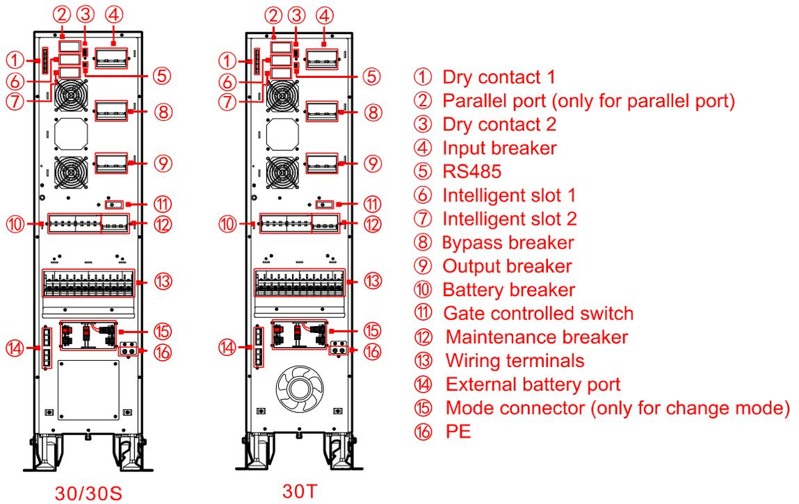
Figure2-8 Structure of 30kVA rear panel
