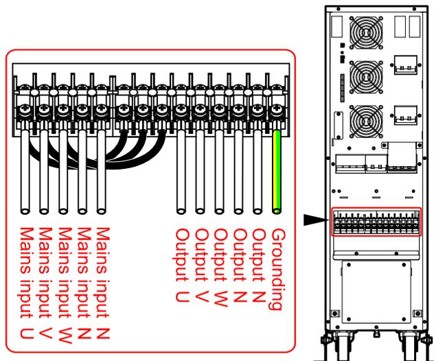
Figure3-14 Wiring diagram of 33 mode
