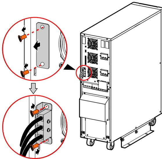
Figure3-28 Extension battery wiring assembly of 10kVA
