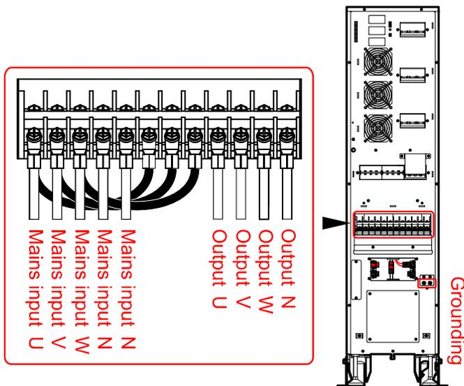
Figure3-22 Wiring diagram of 33 mode
