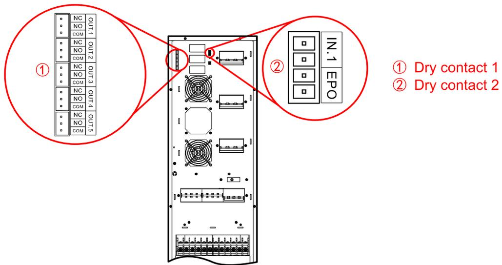
Figure2-11 Dry contact position of 30/30S/30T/40/40S/40T
