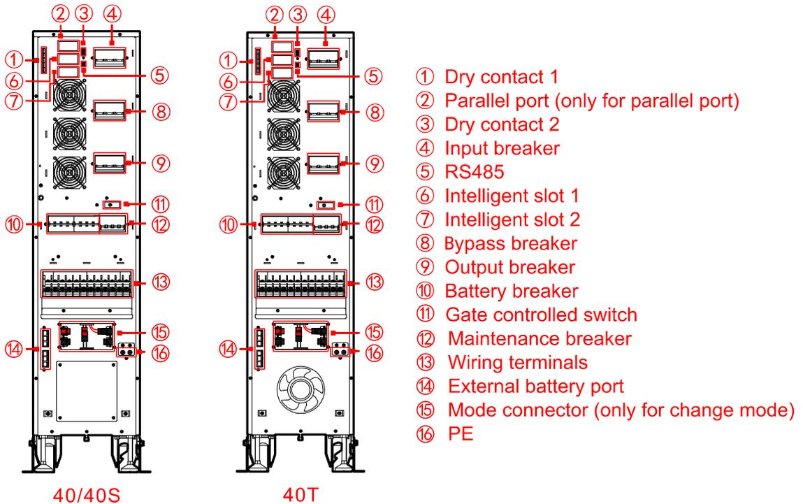
Figure2-9 Structure of 40kVA rear panel
