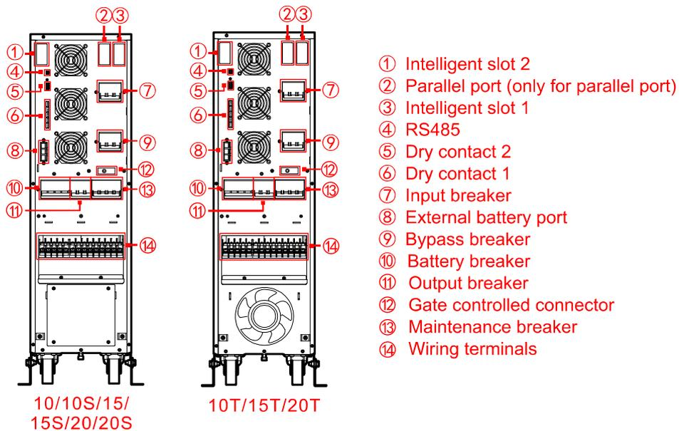
Figure2-7 Structure of 10/15/20kVA rear panel
