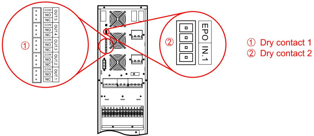
Figure2-10 Dry contact position of 10/10S/10T/15/15S/15T/20/20S/20T
