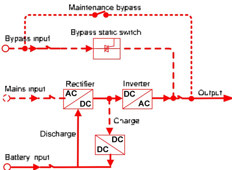
Figure2-14 Battery inverter mode (the thick solid line stands for the energy flow direction)
