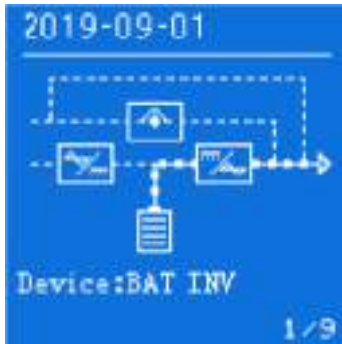
Figure4-5 Battery Inverter Output
