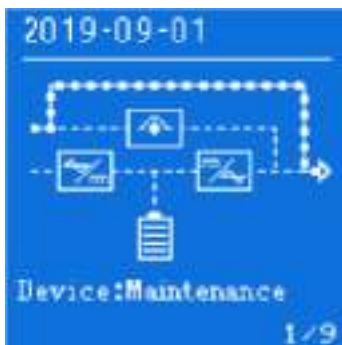
Figure4-7 Maintenance bypass output
