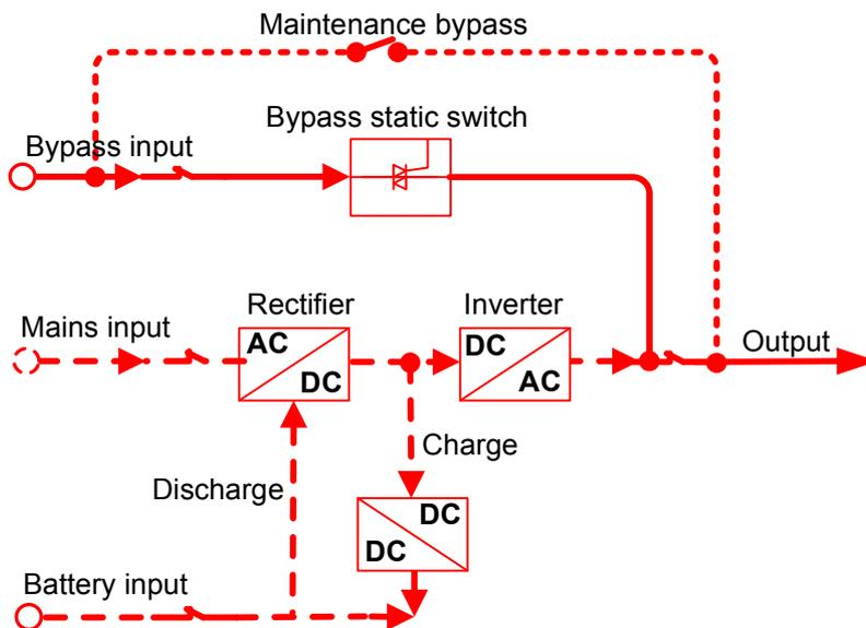
Figure2-15 Bypass power supply mode (the thick solid line stands for the energy flow direction)
