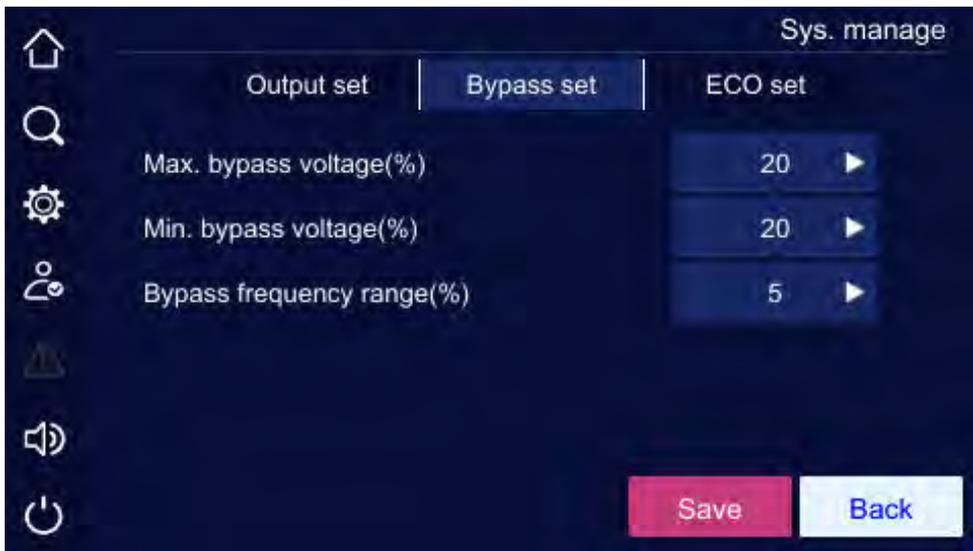
Figure5-25 System manage page 2 of bypass set
