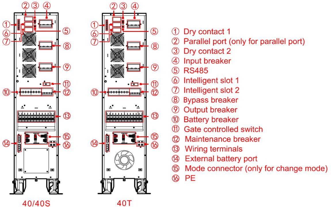
Figure2-9 Structure of 40kVA rear panel
