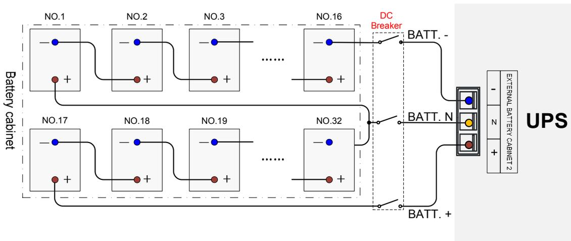
Figure3-25 Wiring diagram 1 of external batteries
