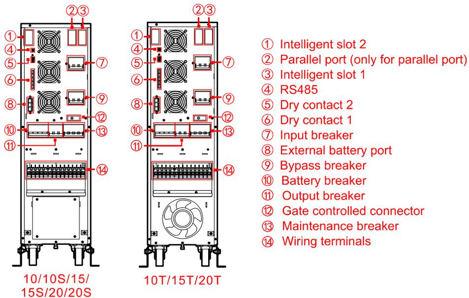
Figure2-7 Structure of 10/15/20kVA rear panel
