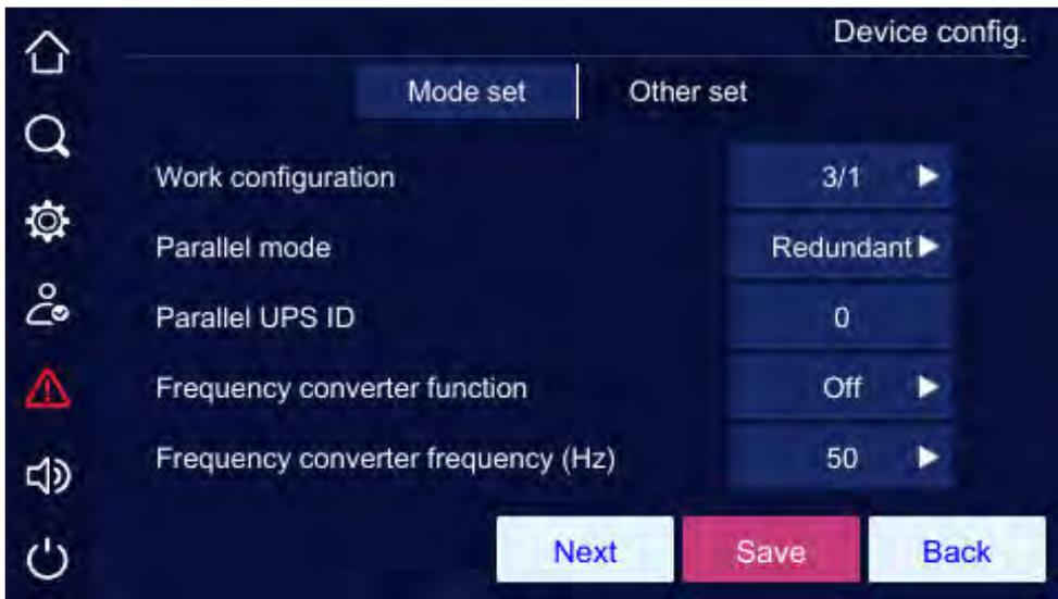
Figure5-41 Mode set page 1 of device configuration
