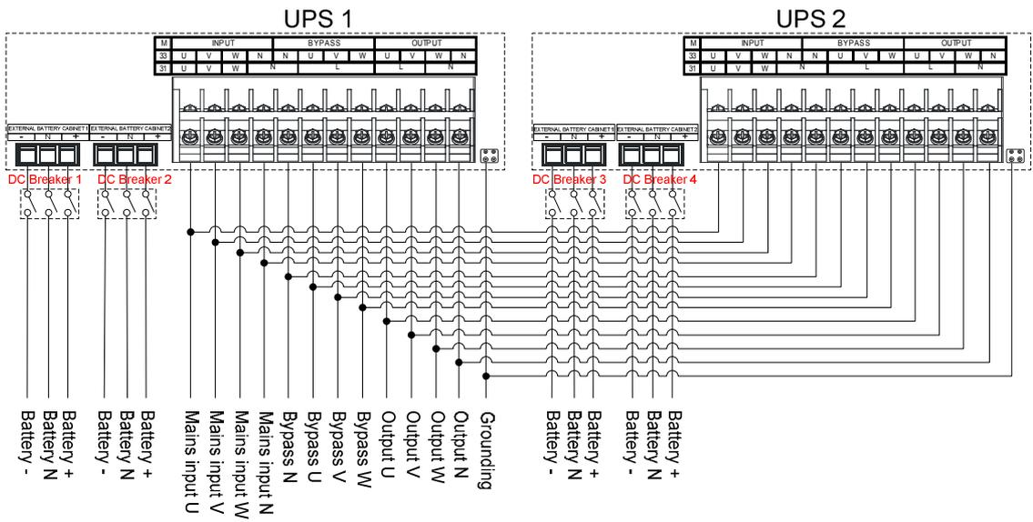
Figure3-32 33 mode parallel system wiring diagram of 30/30S/30T/40/40S/40T
