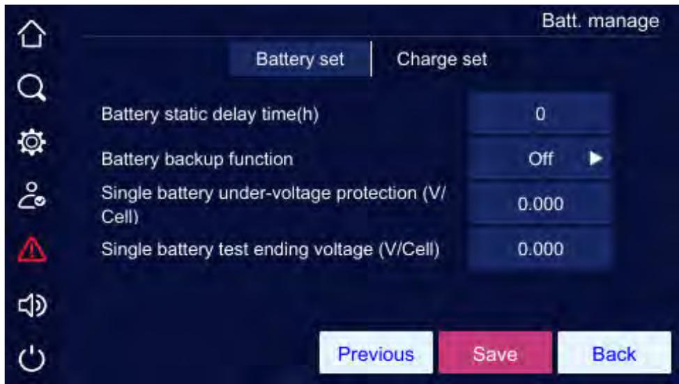
Figure5-30 Battery set page 2 of battery management
