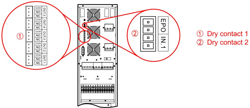
Figure2-10 Dry contact position of 10/10S/10T/15/15S/15T/20/20S/20T
