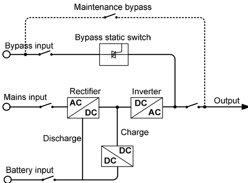
Figure2-12 Work principle diagram
