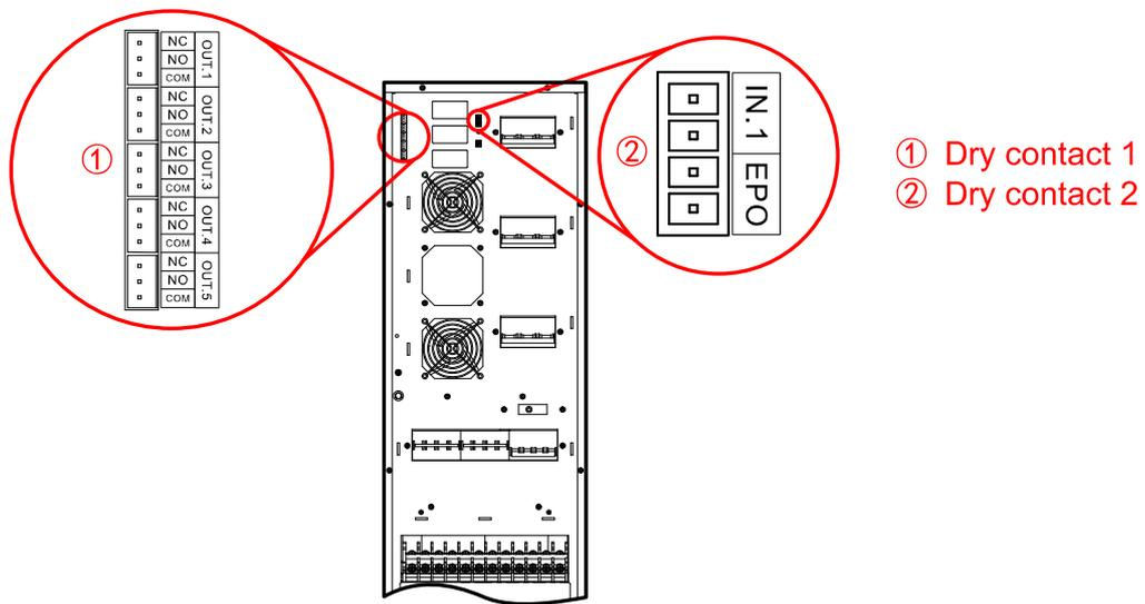
Figure2-11 Dry contact position of 30/30S/30T/40/40S/40T
