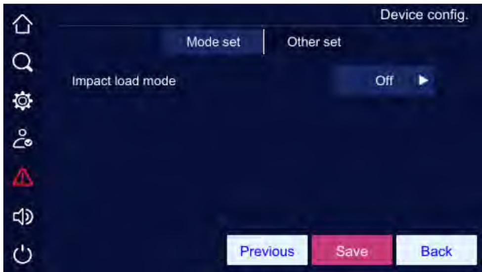
Figure5-43 Mode set page 3 of device configuration
