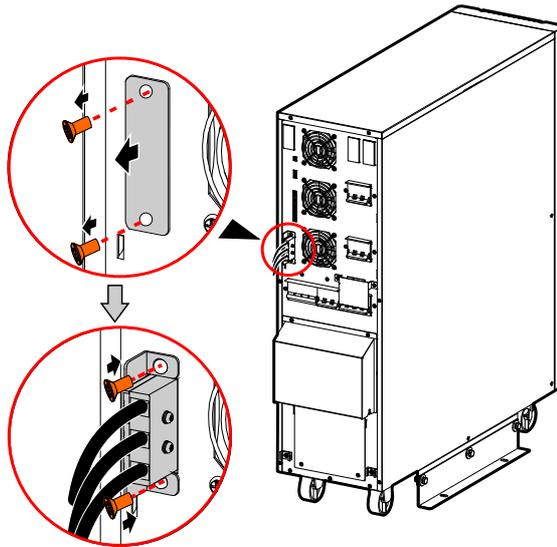
Figure3-28 Extension battery wiring assembly of 10kVA
