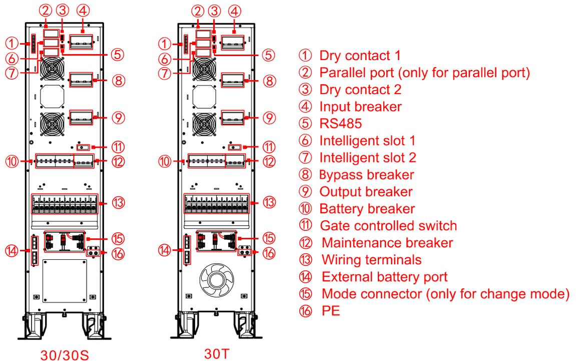
Figure2-8 Structure of 30kVA rear panel
