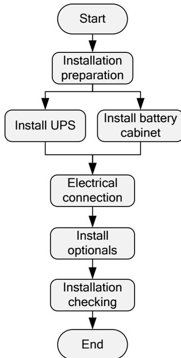
Figure3-1 UPS installation process
