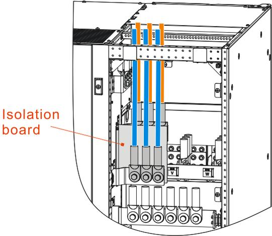
Figure3-32 The PS500KVA、PS600KVA battery wiring diagram
