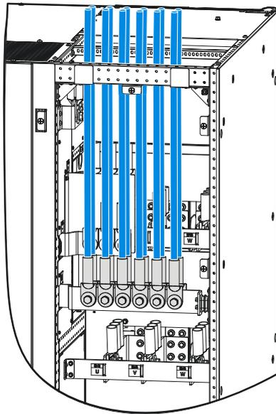
Figure3-33 The PS500KVA、PS600KVA output neutral wiring diagram
