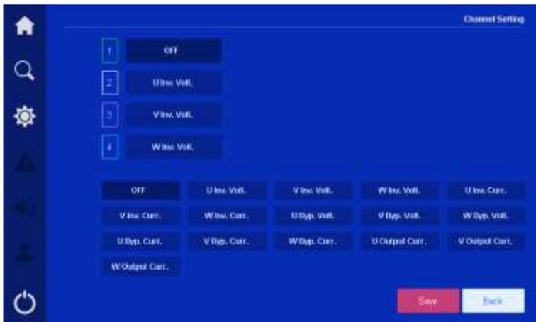
Figure4-24 Channel setting of fault wave page
