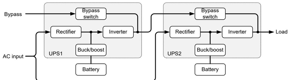
Figure 2-3 Operating principle of series hot-standby system
