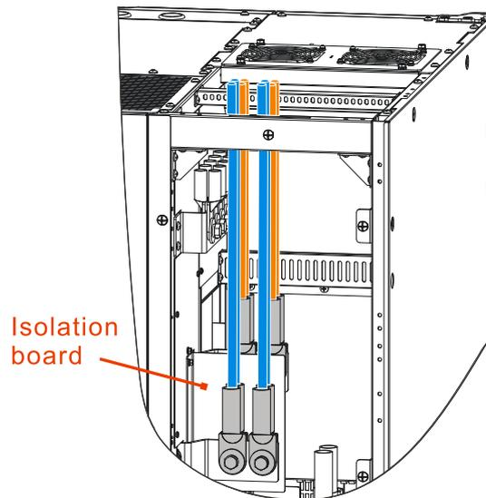
Figure3-23 The PS300KVA, PS400KVA battery wiring diagram
