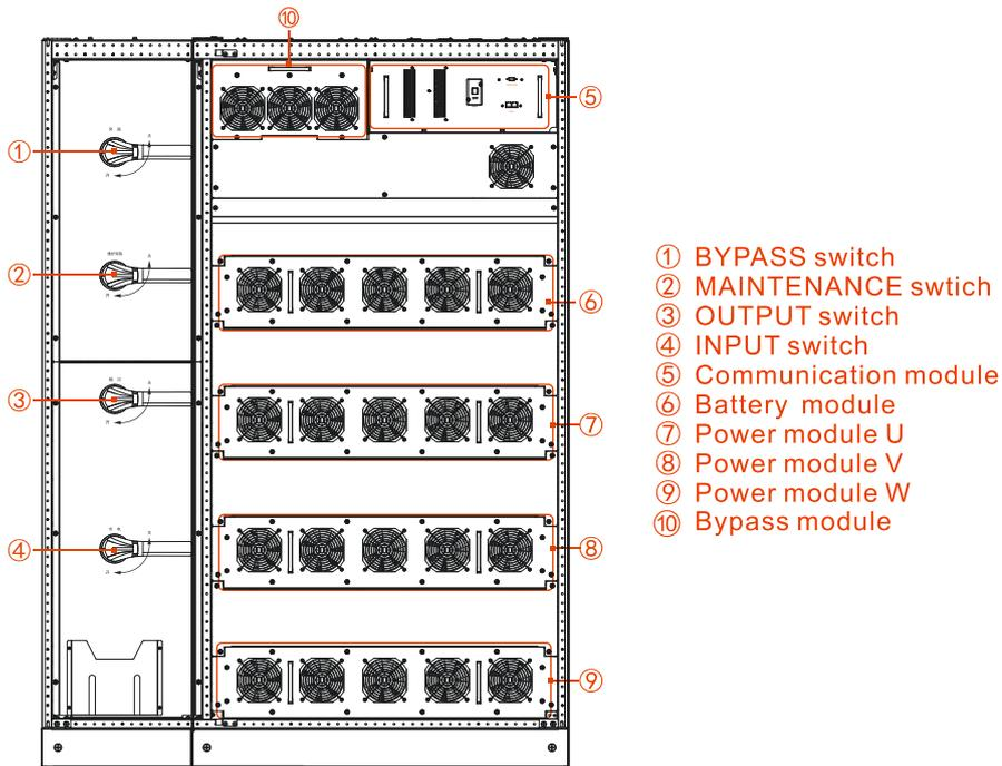
Figure2-11 Structure layout of PS500KVA, PS600KVA (open door)
