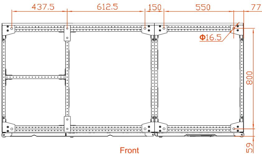
Figure3-13 Pedestal installation size of PS800KVA (unit: mm)
