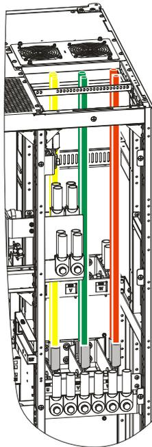
Figure3-20 The PS300KVA, PS400KVA AC output wiring diagram
