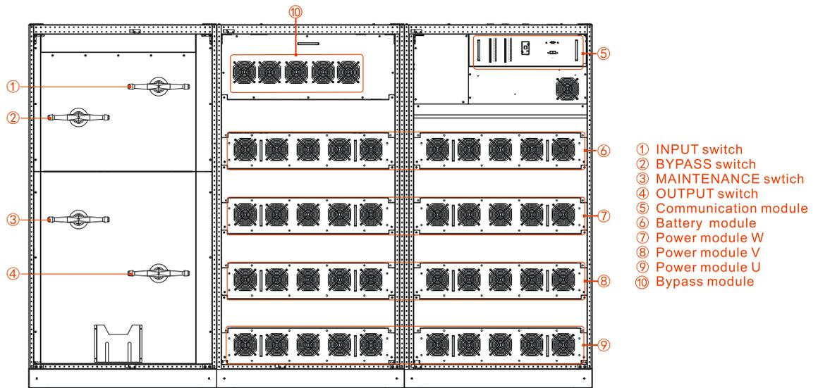
Figure2-13 Structure layout of PS1000KVA, PS1200KVA (open door)
