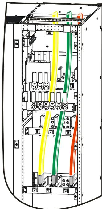
Figure3-30 The PS500KVA、PS600KVA AC input wiring diagram
