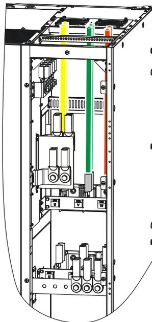
Figure3-19 The PS300KVA, PS400KVA bypass input wiring diagram
