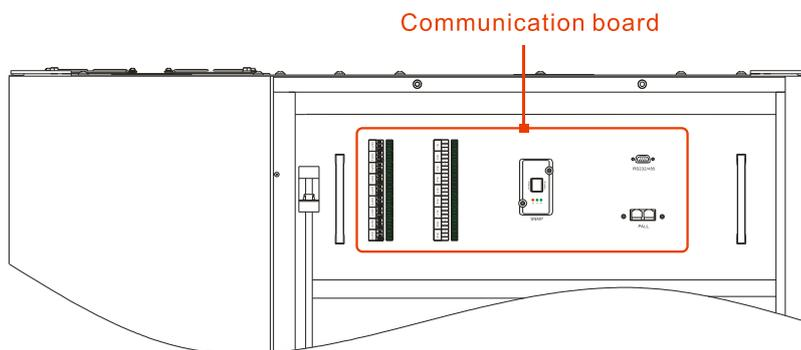
Figure3-25 Communication board of PS300KVA, PS400KVA
