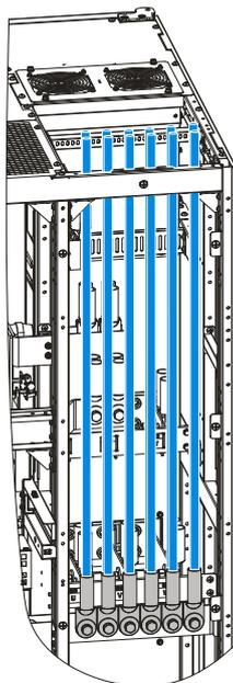
Figure3-24 The PS300KVA, PS400KVA output neutral wiring diagram
