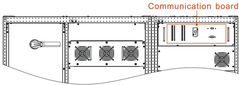
Figure3-43 Communication board of PS800KVA
