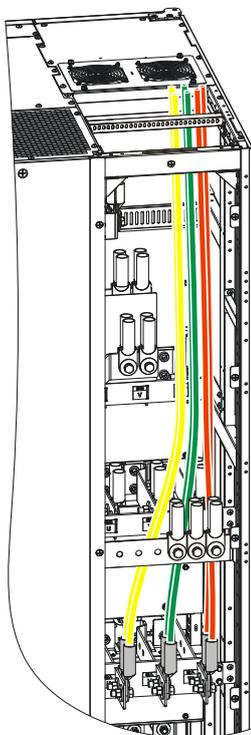
Figure3-21 The PS300KVA, PS400KVA AC input wiring diagram
