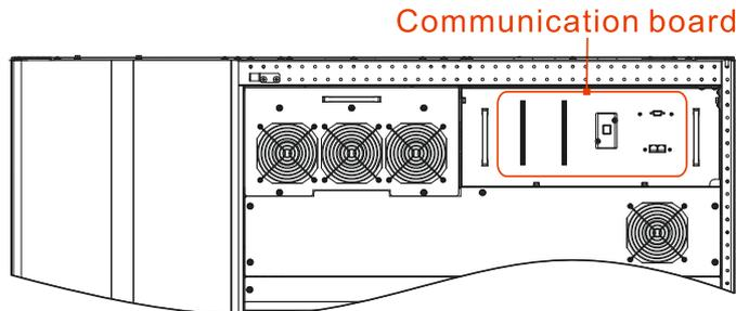
Figure3-34 Communication board of PS500KVA, PS600KVA
