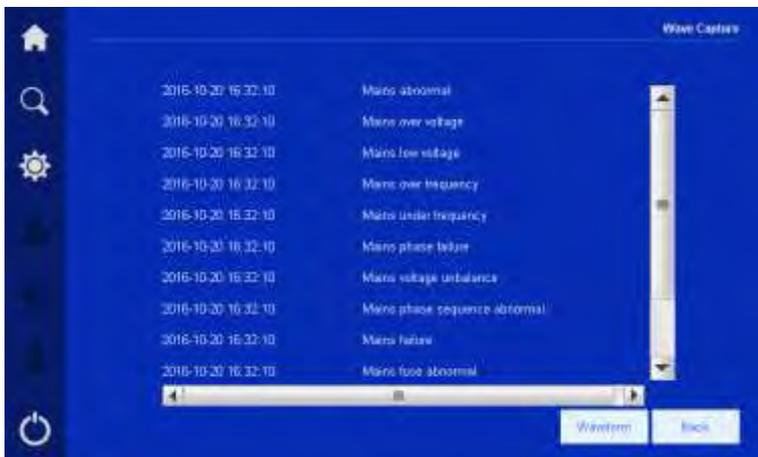
Figure4-22 Corresponding fault details of fault time
