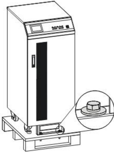
Figure3-5 Bolt position of Three-Phase (10kVA-30kVA) series UPS
