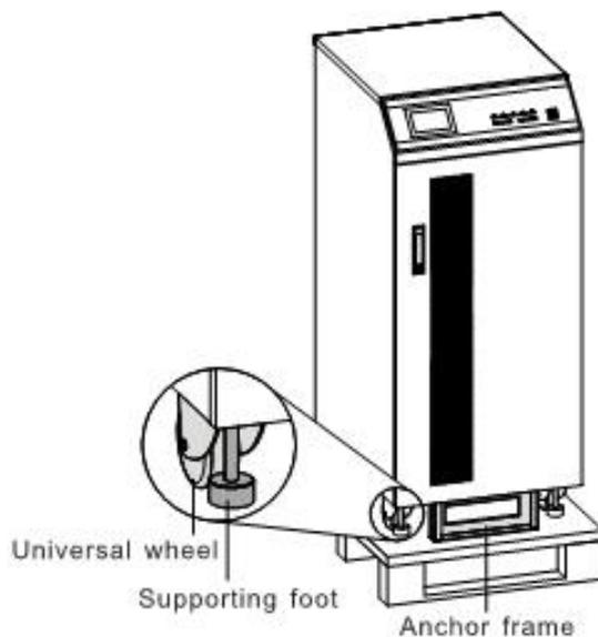
Figure3-16 Rotate four supporting foot
