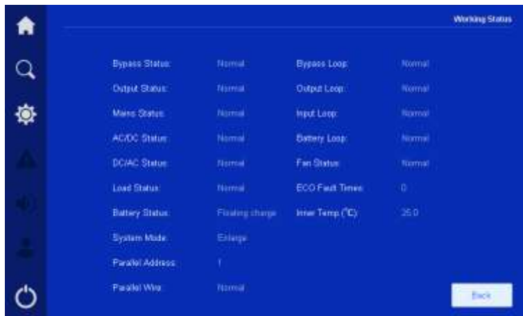
Figure4-19 Working status page (parallel system)
