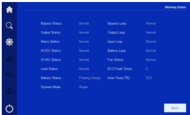
Figure4-18 Working status page (single unit)
