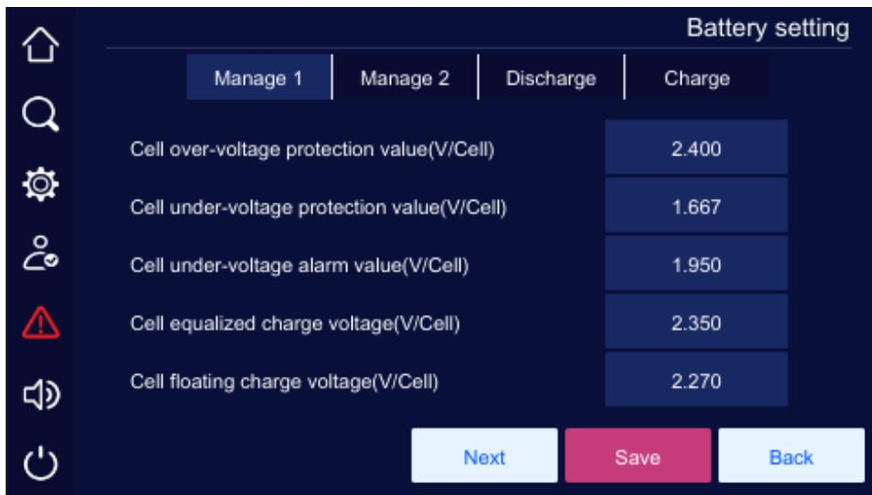
Figure4-21 Battery setting
