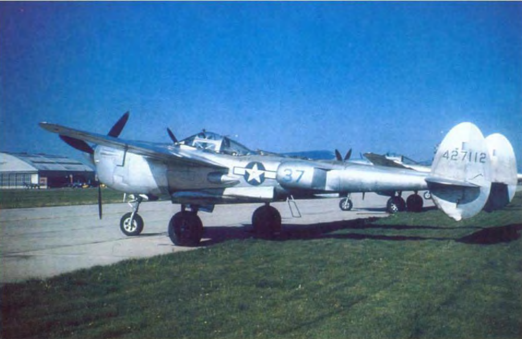
A P-38L-5-LO (44-27112) sits alongside a second Lightning on the ramp at Chanute Army Air Base (AAB), Illinois in 1946. It is plainly marked apart from national insignia, serial number on the tail, and the aircraft-in-group number (37) on the radiator housing. The port radiator door is closed while on the ground. By 1946, the War Department's desire for an all-jet Air Force resulted in the P-38's rapid phase out from US service. (Col O.C. Griffith via David Menard)
