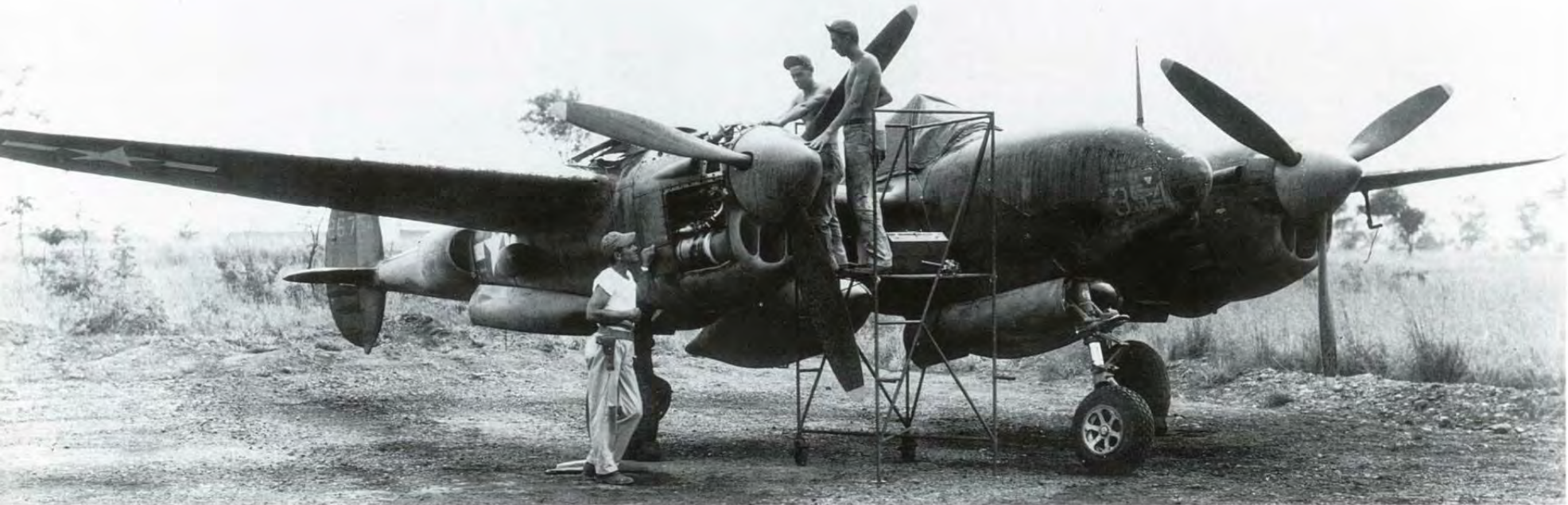
Ground crews service the starboard Allison V-1710 engine of a 25th PRS F-5B-1-LO (42-67354) at San Jose Air Base on Mindoro, the Philippines in late 1944. Two mechanics stand on a metal frame work platform to access the upper engine section. Well-worn nose
