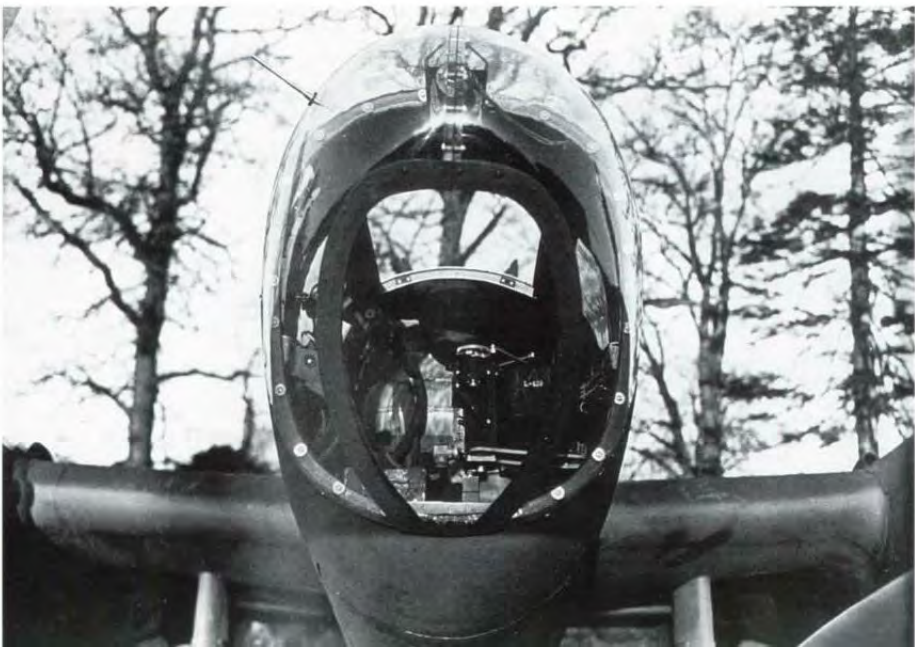
The Norden bombsight was mounted in the port side of the P-38J 'Droop Snoot' nose compartment. An optically flat panel in the bubble allowed for distortion-free sighting of the target. The bombardier entered his cramped station through a hatch in the floor. 'Droop Snoot' P-38Js carried up to 4000 pounds (1814.4 kg) of bombs under the wings. (Lockheed)
