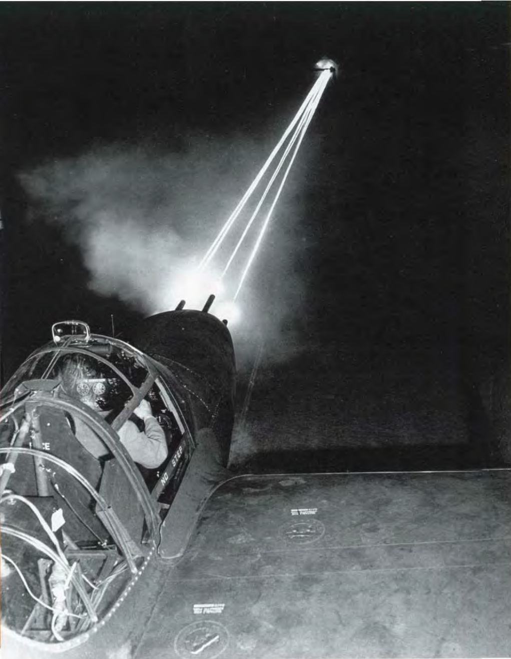
A Lockheed technician fires the P-38F's four nose-mounted .50 caliber (12.7mm) Browning M2 machine guns on a nighttime ground test. This mounting resulted in an almost nonexistent spray pattern to the guns and a high percentage of hits. The wing fillet added to this Lightning variant eliminated elevator buffeting that troubled earlier P-38s. The rear view mirror fitted to all production Lightnings protrudes from atop the canopy. (Lockheed)
