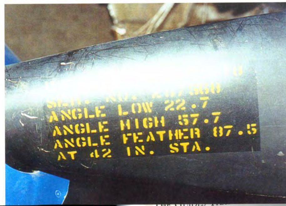
This decal near the propeller hub displays the specifications for its installation in Orange Yellow letters. The three angles of propeller settings – low (22.7°), high (57.7°), and feathering (87.5°) – are also given for the benefit of maintenance crews. This information was displayed on each propeller blade. (Via John Clements)
