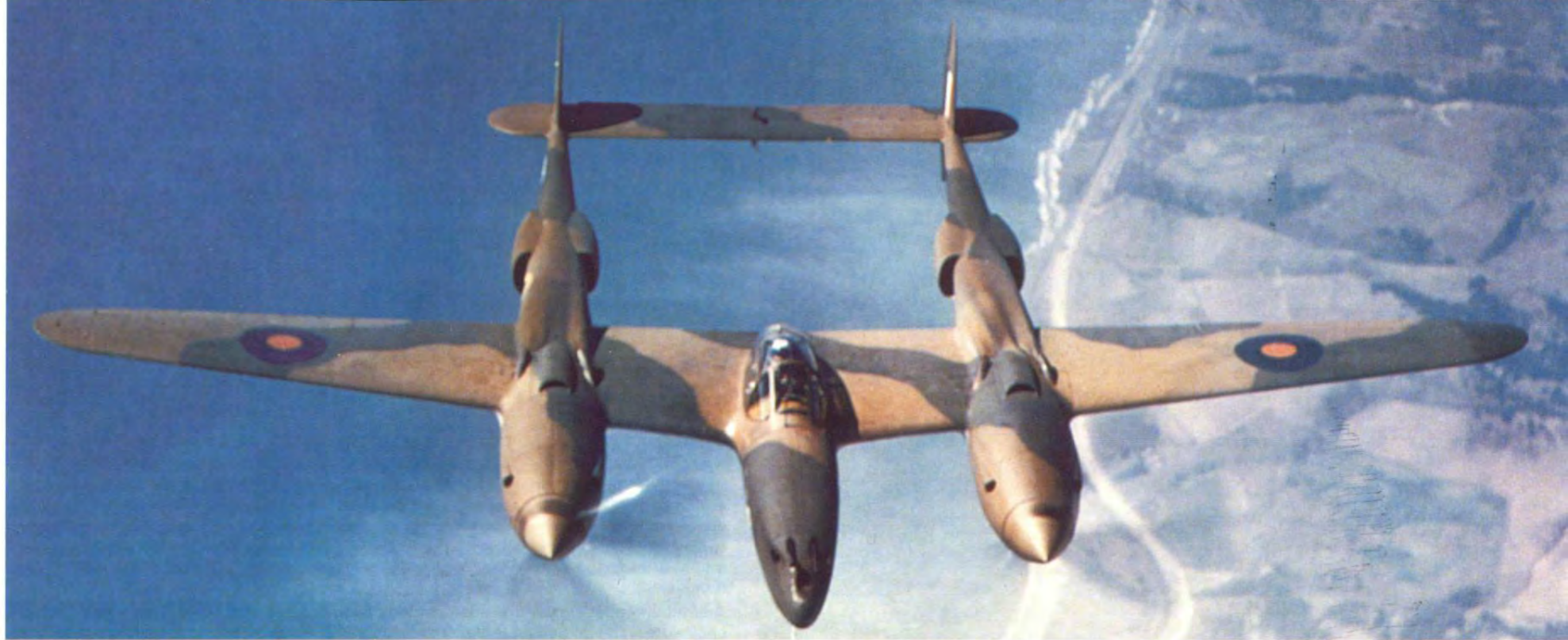
(Above) One of the Model 322 Lightning Mk Is for Britain's Royal Air Force (RAF) flies off the California coast during the late summer of 1941. The fighter's upper surfaces are painted in the RAF camouflage colors of Dark Green (FS34079) and Dark Earth (FS30118), with Sky (FS34504) undersurfaces. The US government would not allow the export of engine superchargers at the time; thus, the Lightning Is were powered by non-supercharged 1090 HP Allison V-1710-C15 engines turning both propellers to starboard. The RAF ordered 143 Lightning Is, but only accepted three aircraft and none of these saw combat. (Lockheed)
