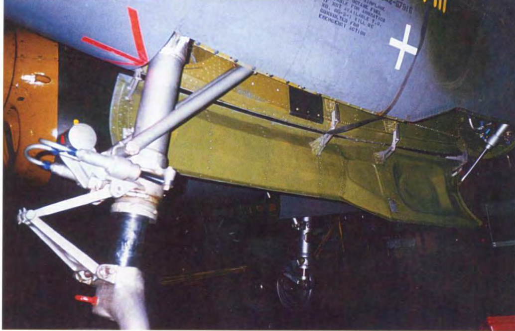
(Above) The P-38 nose gear door had four hinges to starboard and was bulged at the rear for tire clearance. The nose gear fully retracted aft into the gear bay. The gear bay and door interior on this restored P-38J is painted ANA 611 Interior Green (FS34151); however, factory specifications called for Chromate Yellow Primer to be used on these areas. (Keith Melville)
