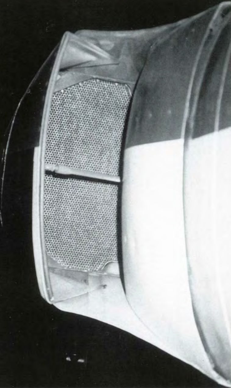
The engine coolant radiator exhaust doors are opened on this statically-displayed P-38. A hydraulic actuator closed the door in flight and opened it while on the ground. A mesh screen covered the radiator exhaust opening to keep out foreign objects, which would otherwise interfere with efficient operation. This opening was found on both the inboard and outboard nacelle sides. (Keith Melville)
