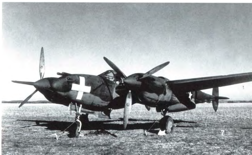
Another 'White Force' P-38D of the 1st PG is parked at Goodfellow Field, Texas in the early fall of 1941. It had taken part in the Louisiana Maneuvers the previous August. This Lightning is fitted with the pointed spinners normally associated with YP-38s. Water-based white paint was used for the cross on the nose, which allowed ground crews to remove the markings after the exercise. (W.L. Bannister)
