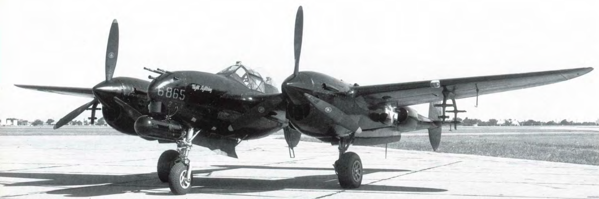
(Above) The first P-38M Night Lightning (44-26865) is displayed after rollout from Lockheed's Dallas modification center in July of 1945. The P-38M was a standard P-38L modified with a Western Electric AN/APS-4 X-band airborne intercept radar housed in a small pod under the nose. The VHF radio mast was relocated from the nose to the port tail boom. The aft fuselage was modified to carry a radar operator immediately aft of the pilot. Lockheed converted 75 P-38Ls into P-38Ms in mid-1945. (Lockheed)
