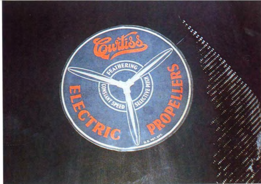
Curtiss Electric propeller decals were applied onto factory fresh P-38s, approximately halfway down the length of each blade. This decal and the surrounding blade surface display some signs of wear. Most propeller decals were removed in combat by the high propeller speeds, weather, or environmental conditions, especially in the Pacific Theatre. (Via John Clements)
