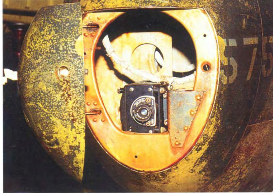
The P-38-LO through P-38J had a gun camera mounted in the nose. This motion picture camera recorded the results of firing runs for confirmation of victories and tactical study. Access to this device was through the opened nose cap, which was hinged to starboard. The P-38L had the gun camera moved to the port wing pylon, where it was less prone to blurred pictures. (John Clements)
