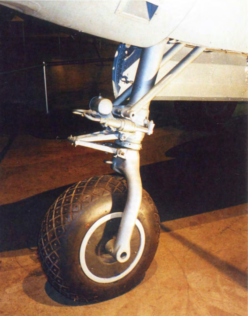
Most early P-38s had hubcaps fitted to the nose landing gear wheel to keep dirt out of the wheel. Many Lightnings – including this P-38J – had this cap fitted only to the port side, where the gear strut connected with the wheel. The 27 inch (68.6 cm) diameter tire had a diamond shaped tread pattern, which was one of the most common tread patterns used. Lack of hydraulic pressure resulted in full compression of the oleo (shock absorbing) inner strut. (Author)
