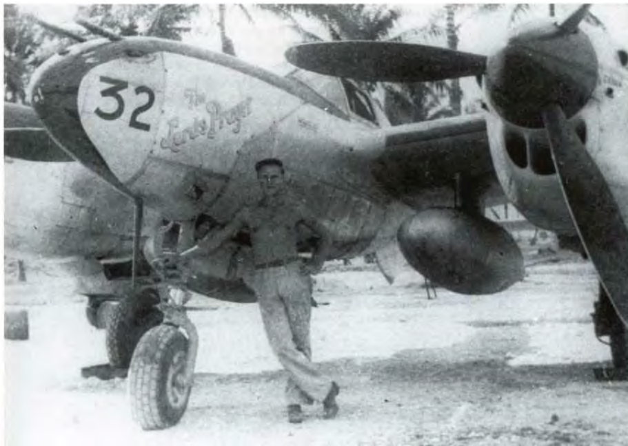
Sgt Harry Kawaski, a 347th FG armorer, stands by The Lords Prayer , an early P-38J assigned to the Group's 339th FS on Leyte, the Philippines in early 1945. This Lightning is equipped with 165 gallon (624.6 L) underwing drop tanks, which were commonly carried by all P-38s in the Pacific Theatre. The color of the nose trim and propeller spinners is unknown. (Richard Schulenberg)
