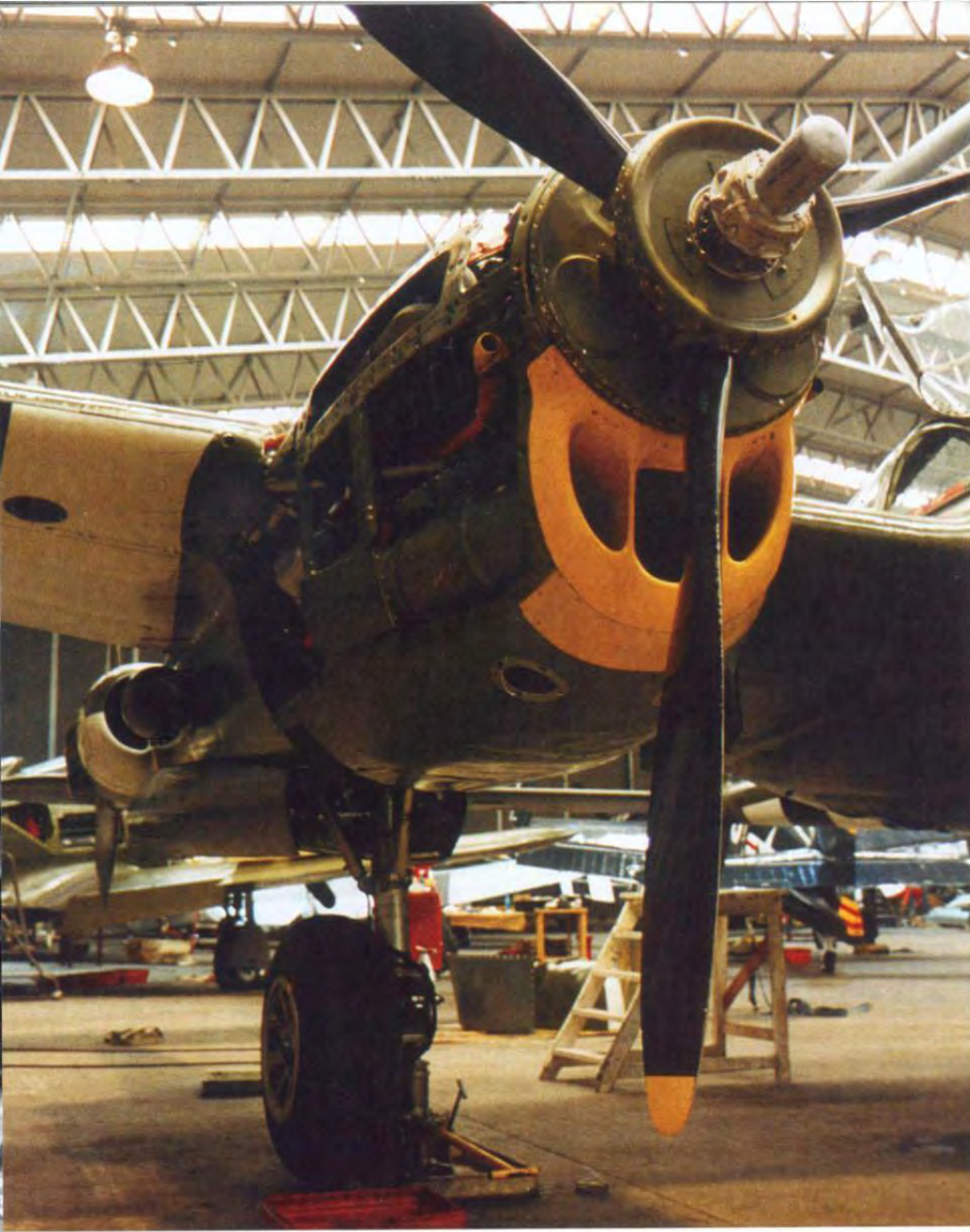
The starboard Curtiss Electric C532D propeller is fully feathered on this P-38J at Duxford, England. A pilot usually employed this 87.5° setting when the engine was out. Placing the propeller blades into a 'knife-edge' direction into the air stream prevented the propeller from 'windmilling,' which resulted in unnecessary drag upon the aircraft. From late 1941, P-38 propeller blades were Flat Black (FS37038) with Flat Orange Yellow (FS33538) tips. (Keith Melville)
