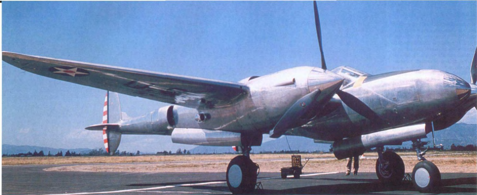
(Above) One of the 13 YP-38s is parked on the Lockheed ramp in late 1940. This service test model differed from the XP-38 prototype in several ways. These included the newly designed engine oil coolers, which were faired into the underside of the forward engine nacelles. The coolant radiators on the aft portion of the engine nacelles were also enlarged on the YP-38. This variant introduced three-bladed Curtiss Electric propellers that turned outboard to improve airflow over the tail. Turning the propellers were two 1150 HP Allison V-1710F engines. (Lockheed)
