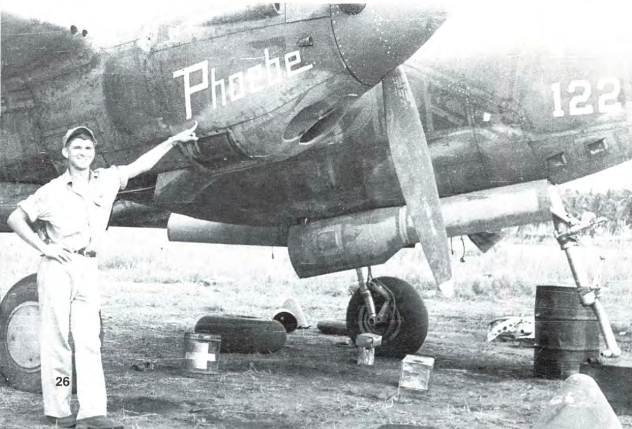
(Above Left) A 431st FS, 475th FG P-38F (132) is parked on 12 Mile Strip near Port Moresby, New Guinea in August of 1943. This Lightning – the first operational fighter aircraft with tricycle landing gear – has a greater nose-high ‘stance’ on the ground, due to having its nose-mounted guns and ammunition removed. The 475th FG was the top scoring P-38 unit during the war, recording 540 victories between 16 August 1943 and 28 March 1945. (Vincent Straus)
