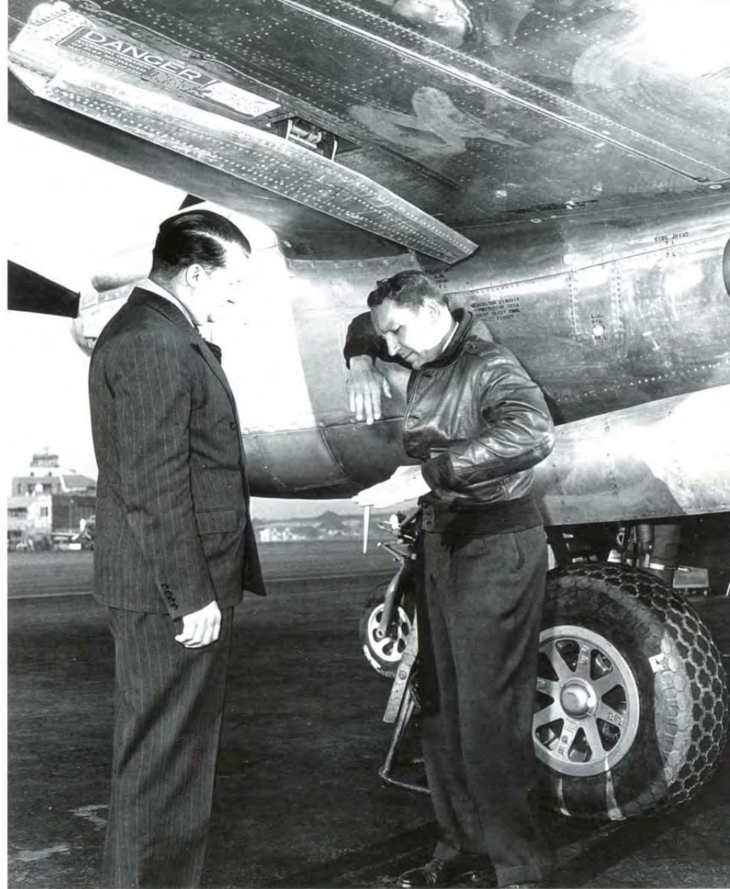
P-38 designer Clarence L. 'Kelly' Johnson (left) and Lockheed chief test pilot Milo Burcham discuss the new compressibility or dive recovery flaps just above their heads. Burcham's hand gestures showed Johnson what happens when these electrically-operated flaps were deployed. The dive flaps were introduced on the P-38J-25-LO and were standard on subsequent variants. They restored lift to P-38s that otherwise stalled and became uncontrollable, particularly at low altitude. The dive flaps reached 35° deflection in only one second. (Lockheed)
