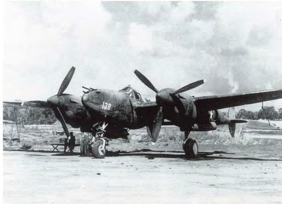
(Above Left) A 431st FS, 475th FG P-38F (132) is parked on 12 Mile Strip near Port Moresby, New Guinea in August of 1943. This Lightning – the first operational fighter aircraft with tricycle landing gear – has a greater nose-high ‘stance’ on the ground, due to having its nose-mounted guns and ammunition removed. The 475th FG was the top scoring P-38 unit during the war, recording 540 victories between 16 August 1943 and 28 March 1945. (Vincent Straus)
