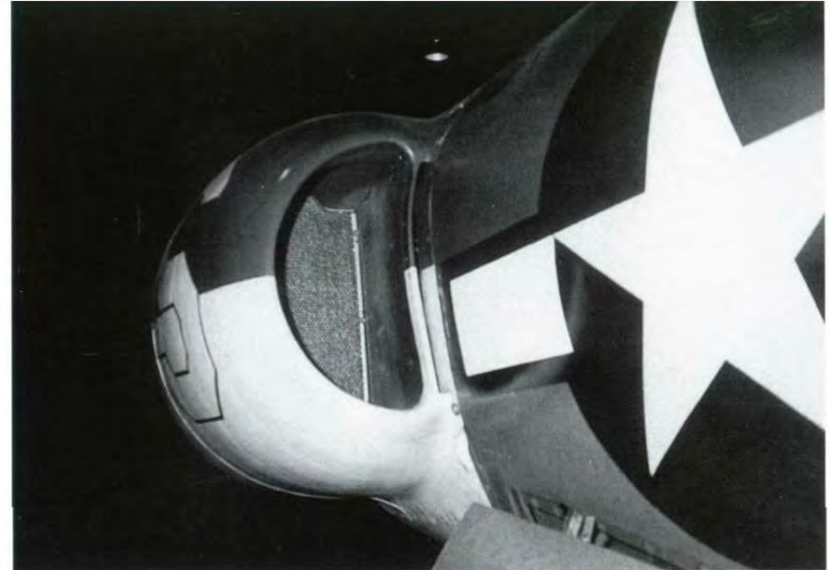
Engine radiator intakes flanked both engine boom sides immediately aft of the main landing gear bay. The semi-circular openings collected air for cooling the radiator, where heated engine coolant was circulated. An anti-foreign object screen is placed inside the intake. P-38Js and later variants featured radiators which were larger, yet more aerodynamically efficient than those fitted to earlier Lightnings. (Keith Melville)
