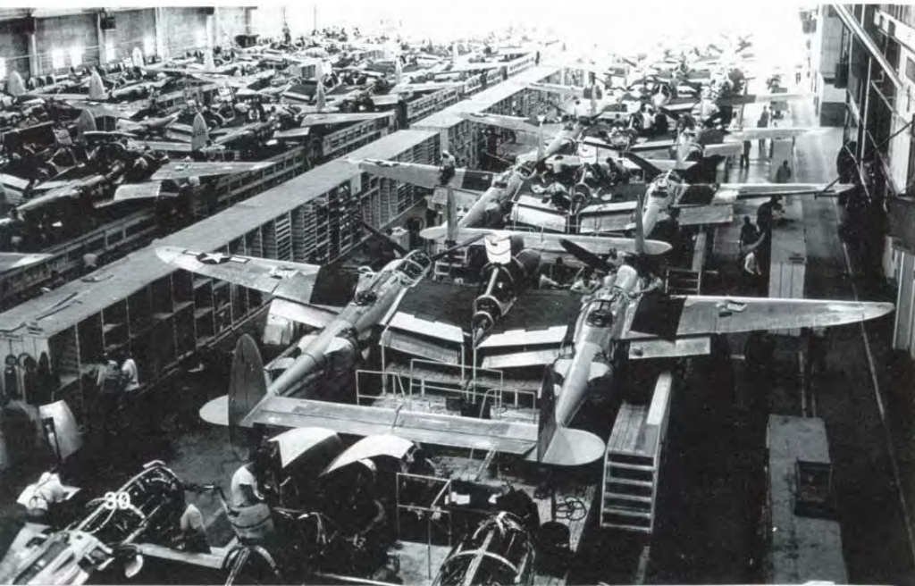
Three columns of P-38Js undergo final assembly at Burbank in August of 1944. The flaps are fully lowered during this stage of production, when there is no hydraulic pressure on these surfaces. Dark covers placed over the wings prevent the shoes of workers and mechanics from scuffing the natural metal surface. The USAAF ended the requirement for camouflaging most new production combat aircraft in August of 1943. (Lockheed)
