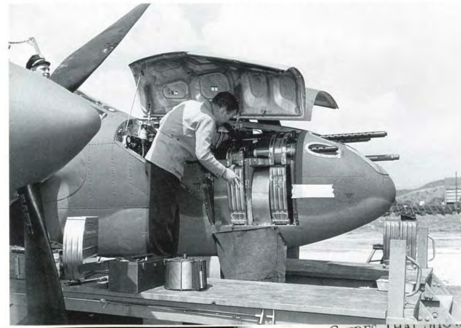
A Lockheed armorer pushes a loaded 500-round .50 caliber ammunition canister back into position. The small rotary 'drum' on the workbench was a 150-round 20mm ammunition canister. Both the gun bay door interiors and the ammunition bins were natural metal, while the gun bay itself was painted Chromate Yellow Primer. A rod extended from the aft bay section kept the inward-hinged gun bay doors opened for servicing. (Lockheed)
