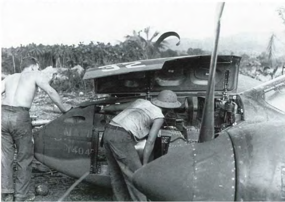
Lockheed armament technicians load .50 caliber ammunition belts into an ammunition bin on a P-38J in 1944. Metal links held the rounds together until they were chambered and fired from the weapon. Each .50 caliber ammunition canister held a total of 500 rounds. Expended ammunition casings were ejected through small chutes cut into the nose undersurface. (Lockheed)
