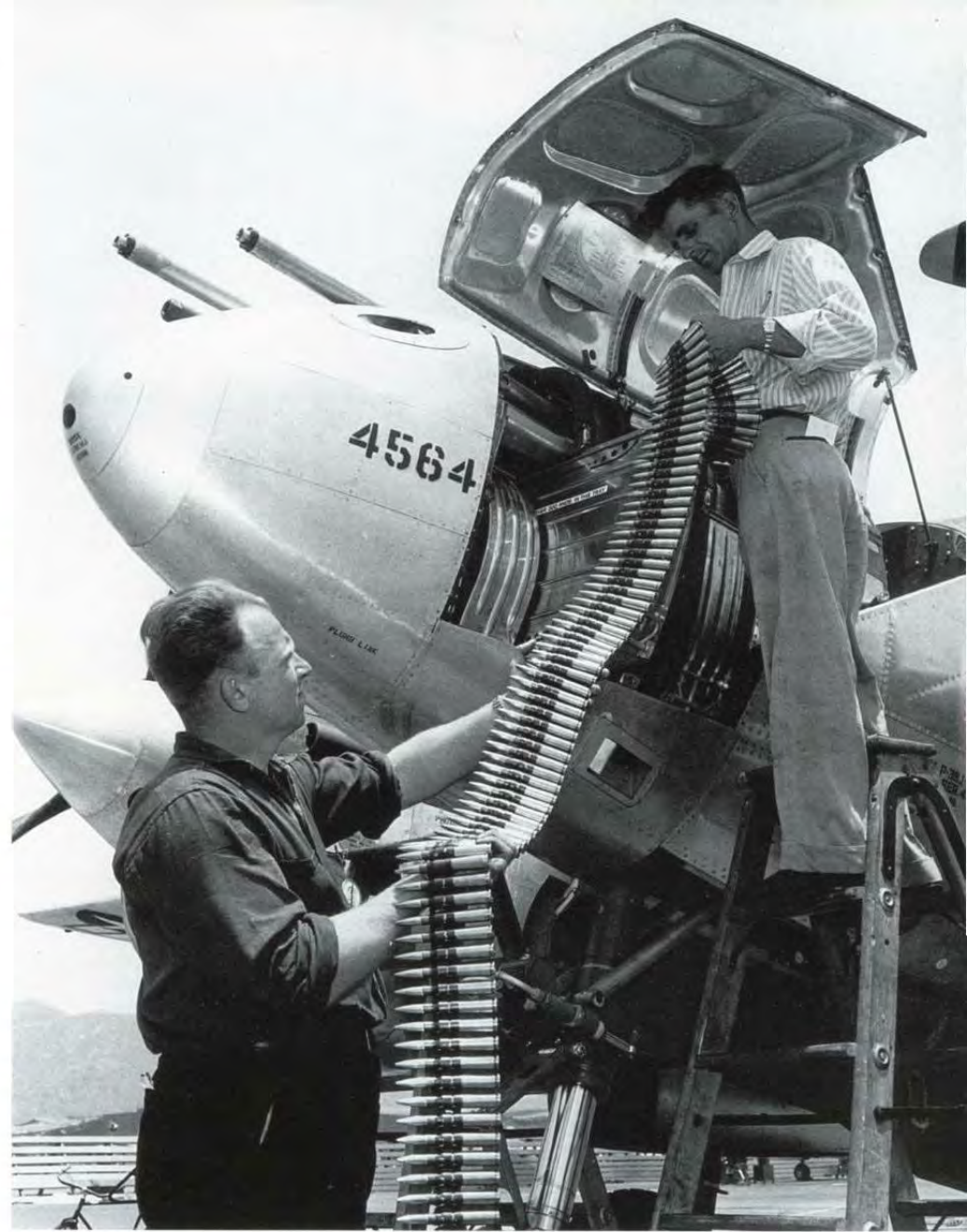
Lockheed armament technicians load .50 caliber ammunition belts into an ammunition bin on a P-38J in 1944. Metal links held the rounds together until they were chambered and fired from the weapon. Each .50 caliber ammunition canister held a total of 500 rounds. Expended ammunition casings were ejected through small chutes cut into the nose undersurface. (Lockheed)
