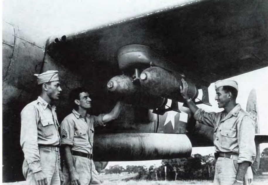
This 82nd FG P-38 was field-modified with an outer wing pylon to both port and starboard. Two 500 pound (226.8 kg) bombs are loaded onto this pylon, which could instead carry three 250 pound (113.4 kg) bombs or a drop tank. This freed the standard inner wing pylons for either drop tanks or additional ordnance. The 82nd FG flew from Vincenzo Airfield in Italy in 1944-45. (Lockheed)
