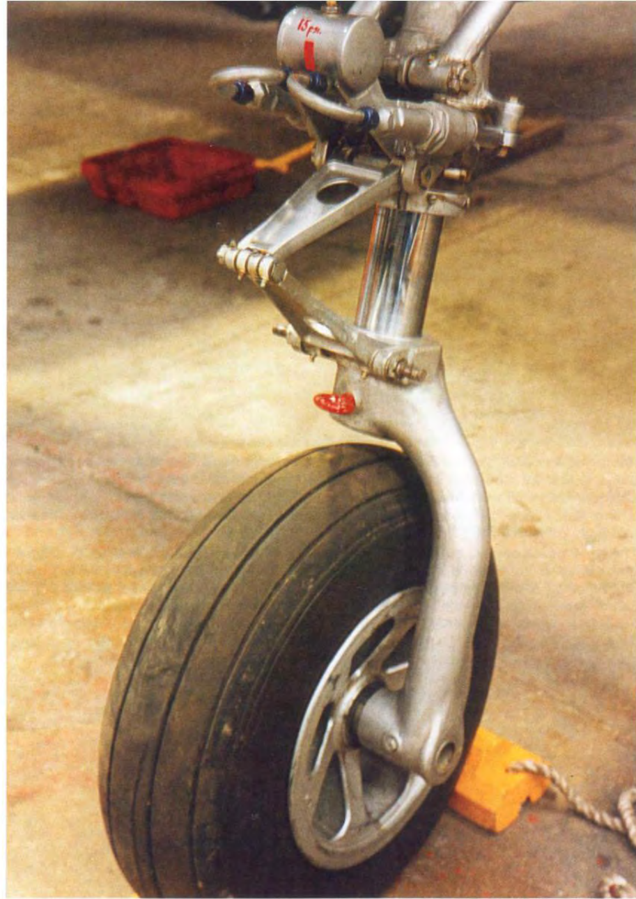
Most later P-38 variants dispensed with the nose wheel hub cap to reduce production and maintenance time. This P-38J is fitted with the circumferential tread design tire that was an alternate to the diamond shaped tread. The chrome plated oleo strut is exposed due to sufficient hydraulic pressure. The red painted tow hook below the oleo was used for towing the Lightning on the ground. (Keith Melville)
