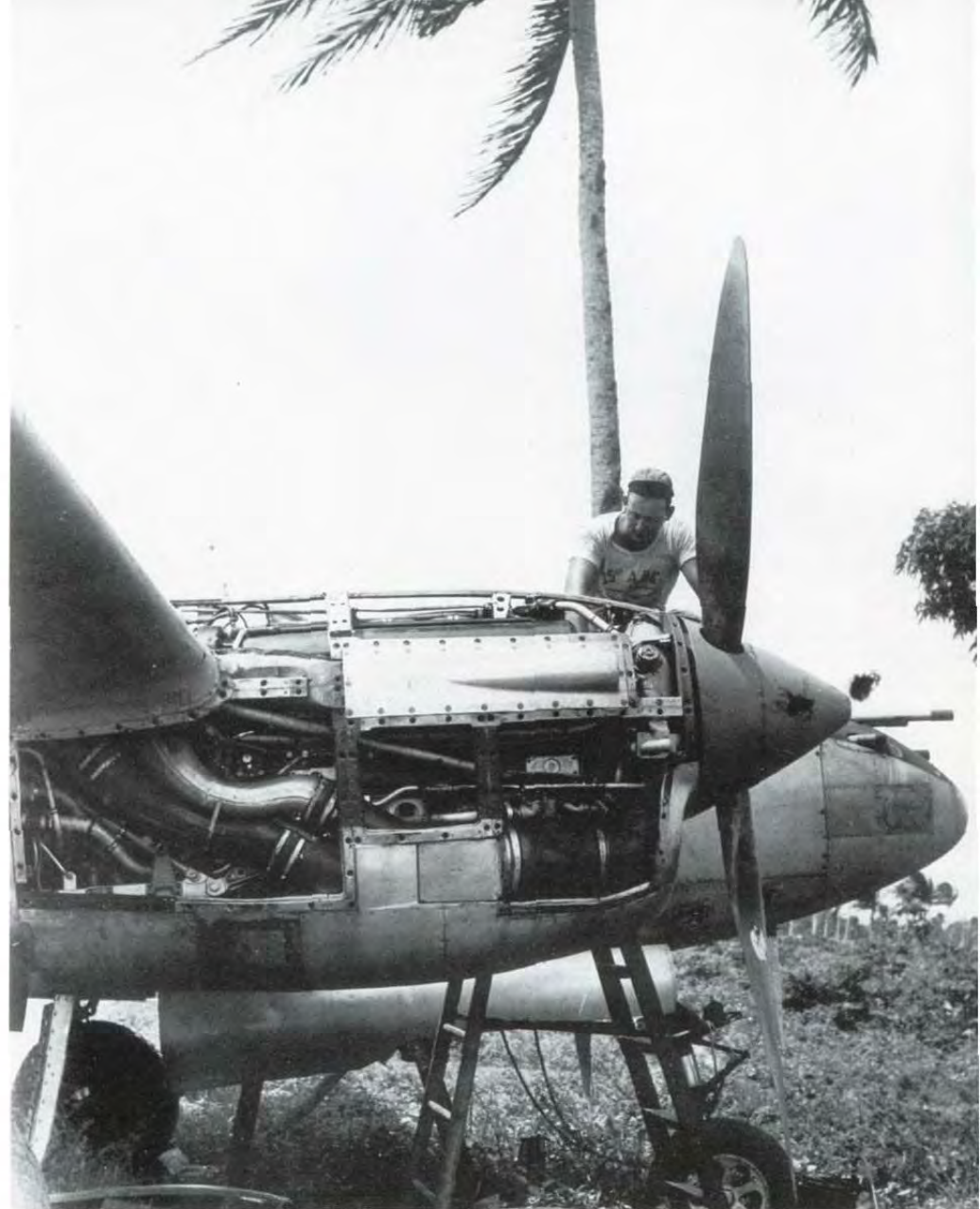
A mechanic services the starboard V-1710 engine of an 8th FG P-38J at the 21st Air Depot facility on Morotai, Netherlands East Indies (now Indonesia) in 1945. Engine cowling panels were removed to service the Allison powerplant, which was overhauled at the depot level every 100 flight hours. Large ducts for the intercooler and carburetor intakes run along the nacelle sides and under the wing leading edge. (Lockheed)
