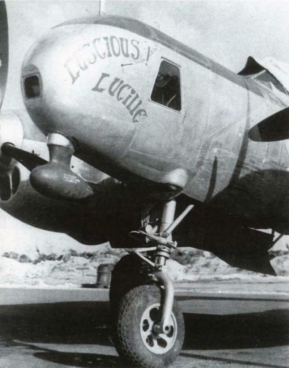
LUSCIOUS ! LUCILLE was an F-5G-6-LO (44-26421) assigned to the 41st PRS at Northwest Field, Guam in 1945. This Lightning is equipped with a football-shaped Automatic Direction Finder (ADF) antenna under the nose. An ADF antenna homed in on radio signals sent by ground stations, which aided the pilot in long-range navigation. The F-5G mounted a forward-looking camera in the nose. Lockheed's Dallas modification center converted 63 P-38L-5-LOs into F-5G reconnaissance aircraft. (James V. Crow)
