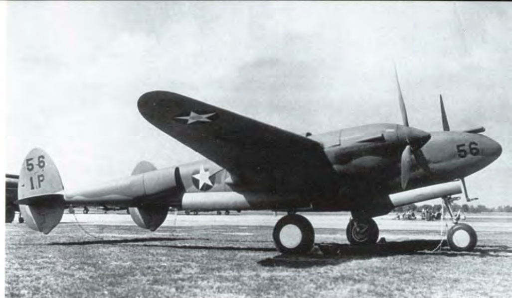
This P-38-LO (56 1P) was assigned to the 1st Pursuit Group (PG) at Selfridge Field, Michigan in the summer of 1941. Essentially the same aircraft as the YP-38, the P-38-LO had the supercharger intake scoop atop the engine nacelle and the new blunt nose propeller spinners. The dual 'guns' in the nose are mockups. The Lightning is painted Olive Drab (FS34087) over Neutral Gray (FS36173). (Art Krieger)
