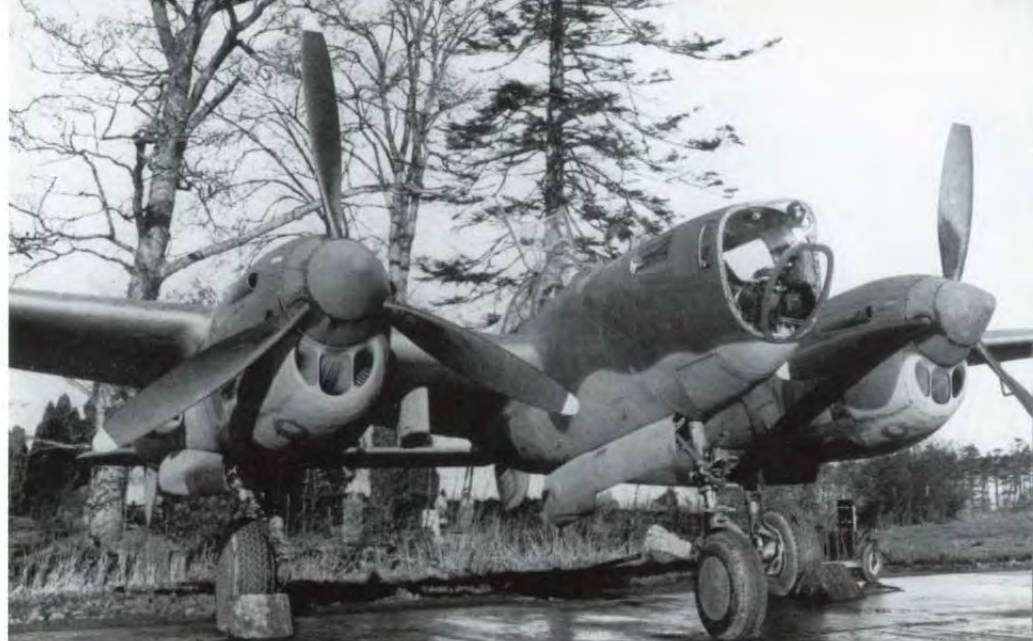
Lockheed converted 23 P-38Js to 'Droop Snoot' configuration in the early spring of 1944. All armament was removed and a Plexiglas bubble was installed in the nose. A bombardier sat in the nose, which was equipped with a Norden bombsight. Lockheed later made 100 'Droop Snoot' conversion kits for field modification of existing Lightnings. (Lockheed)
