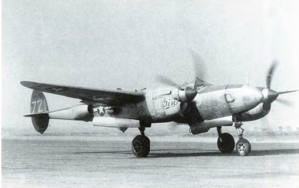
Gin was an F-5E-2-LO (721) serving with the 3rd PRG at Florence, Italy in late 1944. Lockheed's Dallas, Texas modification center converted 100 P-38J-15-LOs to F-5E-2-LO standard. This natural metal Lightning has red and white propeller spinners, while the vertical tail is black with an Orange Yellow number. (USAFM)
