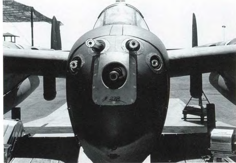
Workbenches and ammunition bins flank the nose of this P-38D undergoing tests at Lockheed's Burbank plant. The four .50 caliber weapons were mounted high on the nose. Early Lightnings were also armed with a 37mm Browning M9 cannon, which was replaced by a 20mm Bendix M1 weapon on the P-38E. A gun camera was mounted in the lower nose below the cannon until it was moved to the port wing pylon on the P-38J. (Lockheed)
