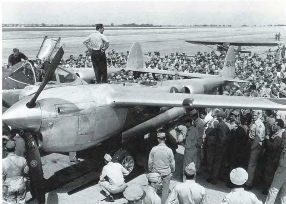
Lockheed Chief Test Pilot Tony LeVier stands on a P-38L at Chico Army Air Field (AAF), California in 1944. He is explaining the differences between this aircraft and all previous P-38 variants. The P-38J and P-38L were almost identical except for the movement of the landing light from inside the outer wing panel to the port wing leading edge. LeVier later put on a flying demonstration of the P-38L, which left all the troops in awe. (Lockheed)
