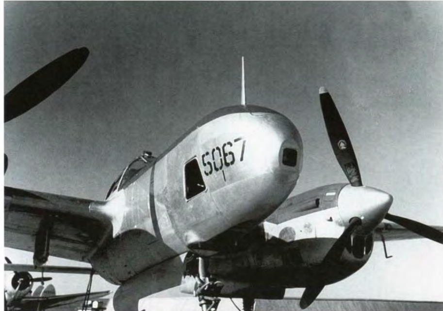
The first F-5G conversion (44-25067) is parked at the Dallas Modification Center after its roll out in 1945. It lacks the ADF antenna later mounted under the nose. The last four digits of the serial number are painted on the nose, ahead of the oblique camera window. F-5Gs were equipped with two oblique and two vertical K-17 cameras, plus an additional forward-looking camera in the nose. (Lockheed)
