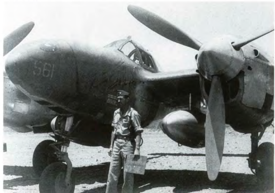
A 34th PRS pilot stands in front of his F-5B (561) at Chateaudun, France in the late summer of 1944. Unusually, this aircraft mated an early F-4A nose onto a P-38J airframe. There was no provision for oblique cameras on this F-5B. Oval patches were riveted over the gun ports. The aircraft is equipped with 165 gallon drop tanks under the wings. (Author's Collection)
