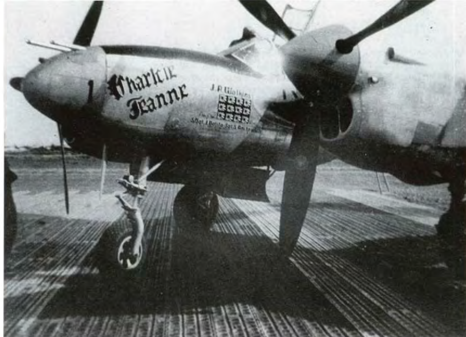
Maj James Watkins flew Charlie Jeanne , a P-38J assigned to the 9th FS, 49th FG at Lingayen, the Philippines in early 1945. Japanese flags indicating Watkins' 12 victories are painted on the nose. His first ten 'kills' came while flying P-38s for the 9th FS in mid-1943. The outer port .50 caliber machine gun was removed from this Lightning and its opening faired over. (Col J. Watkins)
