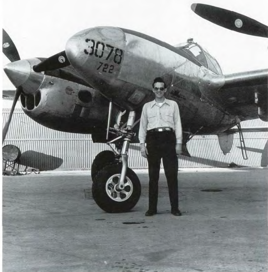
LeVier stands in front of a brand new P-38L-5-LO (722/44-53078) on Lockheed's Burbank ramp in 1944. Guns were not mounted on this Lightning and covers were placed over their openings in the nose. A highly polished oval mirror was mounted on the inboard engine nacelles, just below the antiglare panel. The pilot used this mirror to check the nose landing gear status. P-38Ls had the gun camera moved from the lower nose to the port wing pylon leading edge. (Lockheed)
