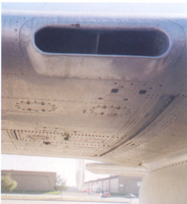
(Left) This large air intake on the leading edge of the wing, outboard of the engine nacelle, provides cooling air for the oil cooler located inside the wing. This area of the wing underside was also strengthened to carry a pair of bomb racks, each capable of holding 100 pound bombs. (Dave Mason)
