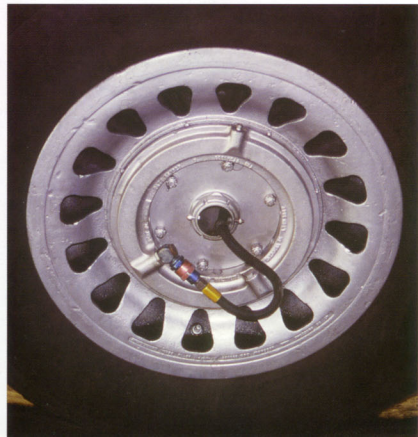
(Left) The flexible brake hose fed the second brake behind the outer wheel face. The main wheels normally did not use cover plates. (Lou Drendel)
