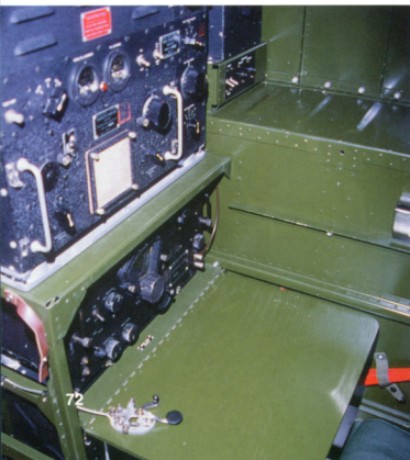
(Left) The navigator was given a folding table for maps and charts work. When the turret was moved forward on the B-25H and J, much of this space was taken up by the turret drive mechanism. Gunships had additional armor plating installed here to protect the cannoneer and the 75mm storage bin. (EAA photo by Phil High)
