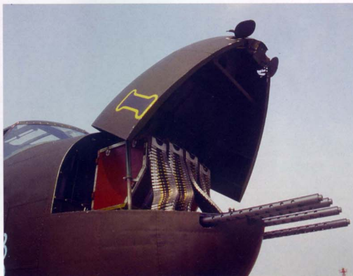
Nose of the well-restored B-25H "Barbie III". The H model was the ultimate strafing version, incorporating up to 10 forward-firing 50 caliber machine guns — four in the nose, four along the fuselage sides and two in the upper turret — and a nose-mounted 75mm cannon. (Lou Drendel)
