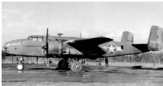
A B-25C-5-NA (42-53357) of the 7th Photo Group at Mt. Farm Airfield, England during early 1944. Worthy of note is the exhaust configuration, one of several tried before the more efficient stacks version led to fairings on the engine cowling. (Robert Astrella via Norm Taylor Collection.)
