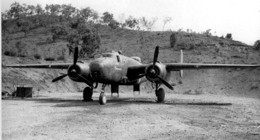
A B-25C, believed to be of the 500th BS, 345th BG, awaits its crew in New Guinea. The lower nose glazing has been altered to accept four additional nose guns. The remaining glazed area has been painted over. The aircraft is also equipped with the early style package guns on the fuselage sides as indicated by the single fairing over both weapons. Both crew hatches, with their retractable steps lowered, are open. Both main wheels are blocked with chocks connected by a rope for rapid removal.
