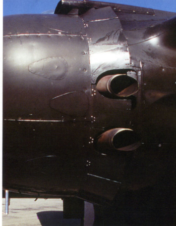
(Left) Engine nacelle of the Canadian Warplane Heritage B-25J. The low profile airscoop on top of the nacelle indicates an early model Bendix-Stromberg carburetor. (Lou Drendel)
