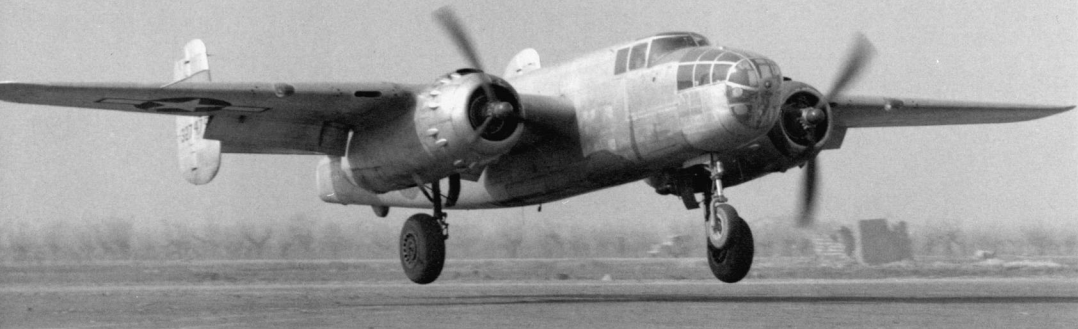
(Above) B-25J-1-NC (43-27475) of the 310th Bomb Group landing at an American base in Tunisia. The absence of all armament indicates that this bomber was used as a high-speed transport and courier. (Norm Taylor Collection.)
