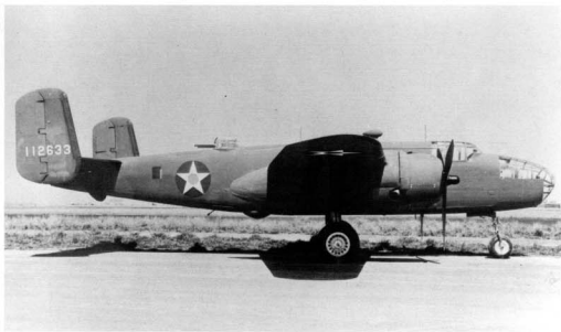
A B-25C (NA-82) fresh off the assembly line in 1942. The ventral turret was retracted into the fuselage, and appears as a slight bulge just under the aft end of the engine nacelle. This early C model was externally identical to the B model. B-25Bs, modified by removal of the ventral turret and addition of over 400 gallons of extra fuel in several tanks, were flown on the Doolittle raid. (North American via Norm Taylor collection)
