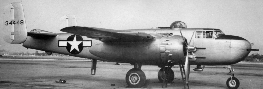
A new B-25H, serial number 43-4448 and fresh out of the factory, sits on the North American ramp on 22 August 1944. A large fairing, covering a K24 camera, has been added to the nose. Cameras this large could take very detailed strike photos or could be used as a forward looking reconnaissance camera. (Norm Taylor Collection.)
