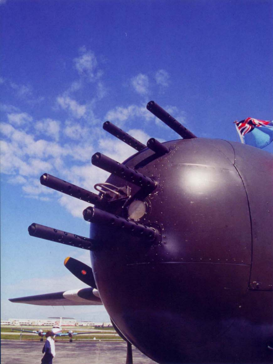
Solid 8-gun nose. The loop antenna mounted between the guns was not on the original version. The first gunships were glass-nosed C and D models packed with additional guns. As the nose was unmanned, the glazing was often painted over. (Lou Drendel)
