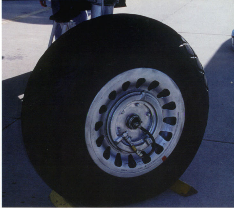
(Left) Narrow hydraulic piping running down the strut fed the dual brakes. One flexible hose ran through the hollow axle to the outside of the wheel. (Lou Drendel)
