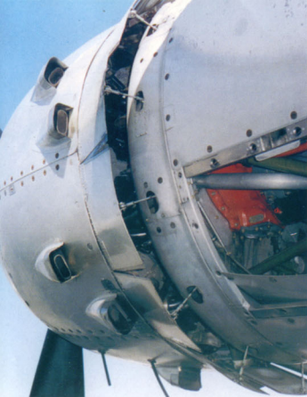
(Left) Cowl flaps almost circled the entire rear edge of the cowl. The flaps were hydraulically actuated using a single pushrod on each flap. (Dave Mason)
