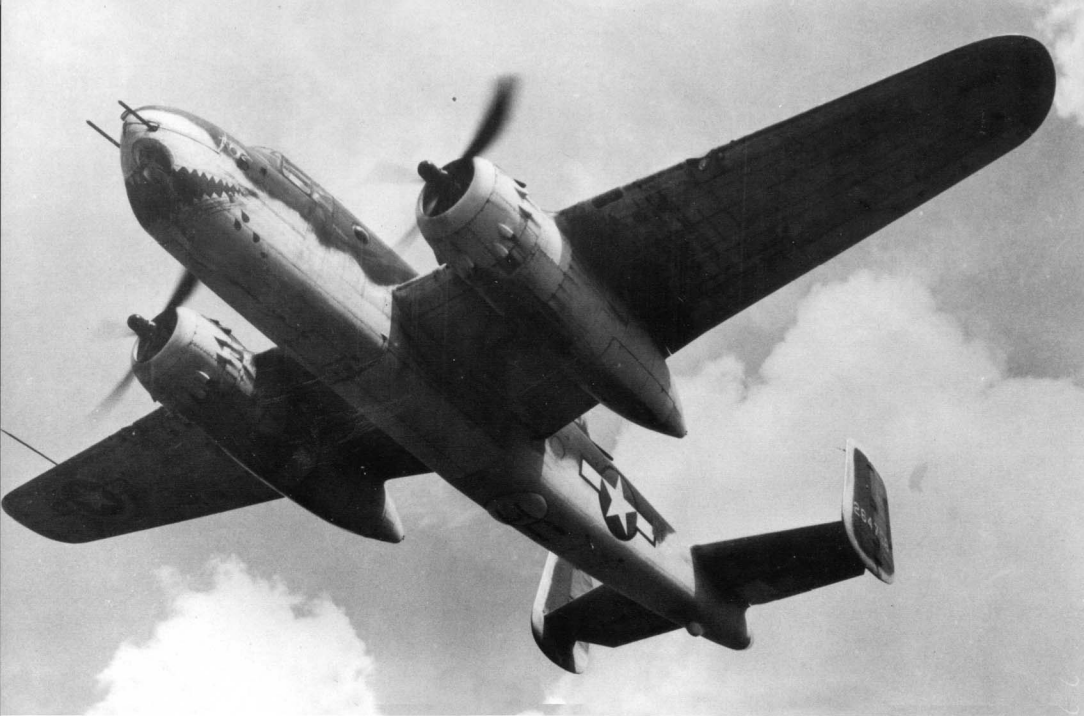
The U.S. Army operated a number of B-25Gs in the submarine-hunting role, flying from bases in the Caribbean and along the U.S. coast. Many were painted in the sea-search scheme of Olive Drab over White. Early B-25Gs were armed with only two .50 caliber machine guns and the 75mm cannon in the nose. (North American)
