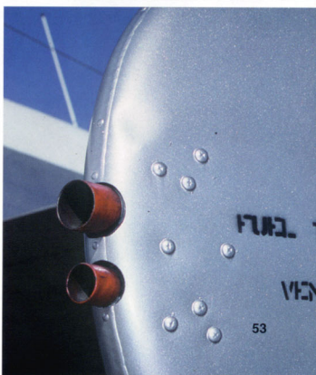
Fuel vent tubes at the rear of the engine nacelles were found all B-25s. Each of the B-25s engines have an independent fuel supply system, interconnected, which allows either engine to operate off of the fuel supply of the opposite engine. (Lou Drendel)
