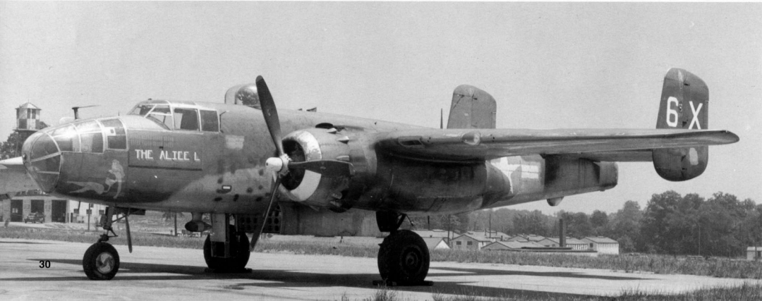
A new B-25H, serial number 43-4448 and fresh out of the factory, sits on the North American ramp on 22 August 1944. A large fairing, covering a K24 camera, has been added to the nose. Cameras this large could take very detailed strike photos or could be used as a forward looking reconnaissance camera. (Norm Taylor Collection.)
