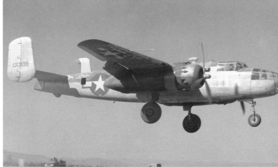
B-25C-1-NC (41-30105) of the 310th Bomb Group on short final to an American base in Tunisia, 1944. The lack of armament indicates the aircraft is likely a squadron hack or transport. The late model exhaust system, characterized by the engine cowling fairings, was the ultimate wartime design. The landing gear has also been painted — probably chromate green (Norm Taylor Collection.)
