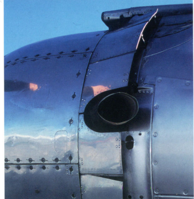
(Right) This exhaust system shows modifications made as a result of problems. The "S" stacks occasionally broke loose from the top cylinder, so a collector ring stack was fitted for the top cylinders, exiting in a single exhaust stack. The lower cylinders retained the original stacks. Cowl fairings were removed and patches installed for the top cylinders, a fairly common modification on post-war B-25s. (Lou Drendel)
