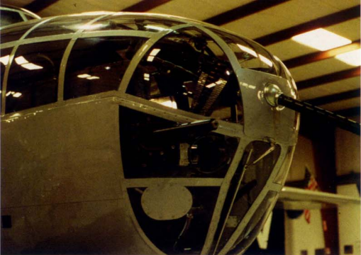
The nose of the Cavanaugh Museum's B-25J has an oval metal panel over the position where an additional fixed forward-firing machine gun would be installed. (Nick Waters)
