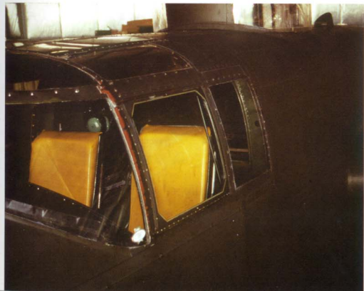
Both pilots were provided a sliding side window for additional ventilation or in the event of extreme misting or icing. (Lou Drendel)
