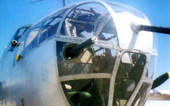
The standard B-25J bomber nose configuration included one fixed, forward firing .50 caliber machine gun and one flexible mount machine gun operated by the bombardier. The large antenna on top of the nose is for modern radio equipment. (Dave Mason)
