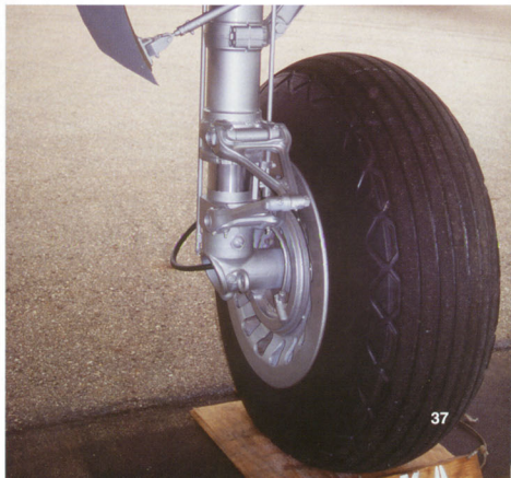
(Left) The flexible brake hose fed the second brake behind the outer wheel face. The main wheels normally did not use cover plates. (Lou Drendel)
