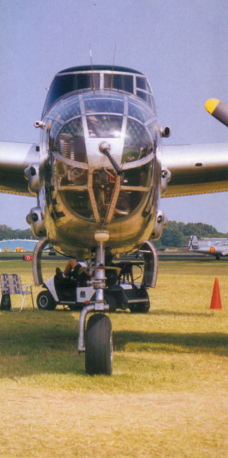
The nose gear is aligned with the centerline of the fuselage. The nosewheel was not steerable, but could caster up to 60 degrees left or right. Normal steering was accomplished via differential braking. In this view, the bomb bay doors are open. (Lou Drendel)
