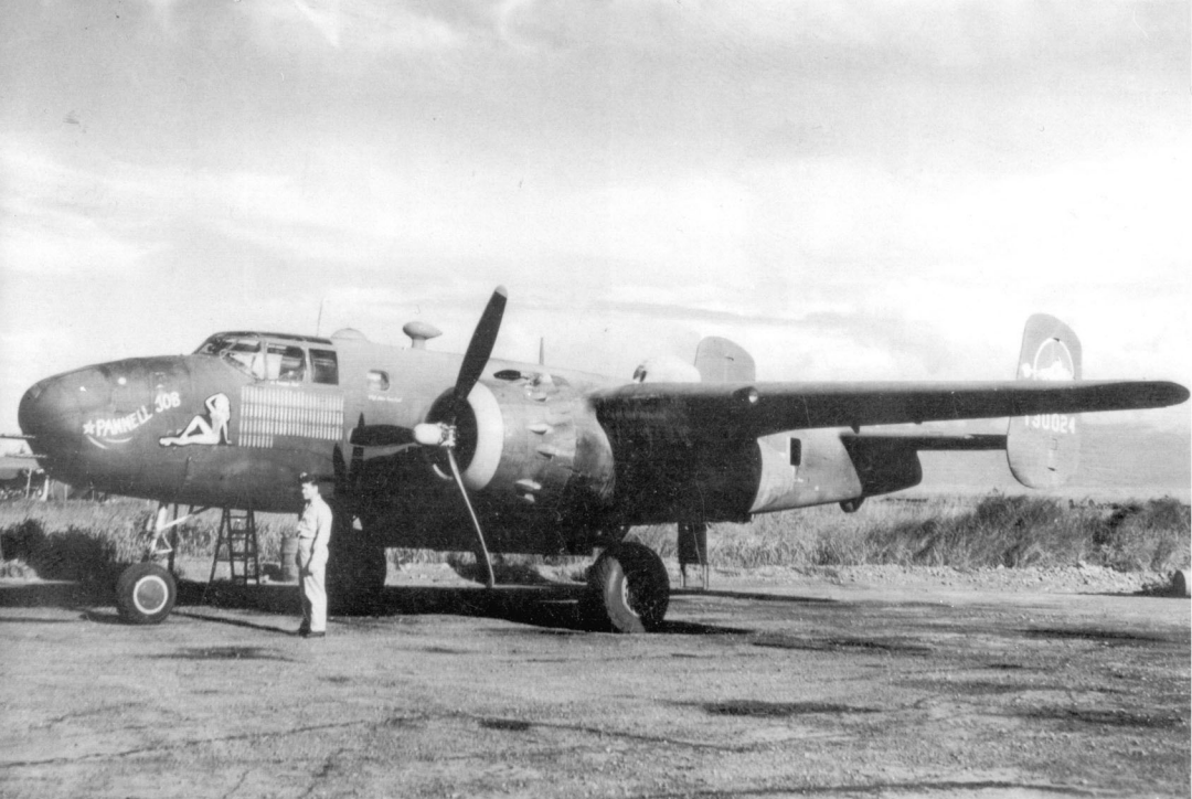
"PANNELL JOB", a B-25C of the 500th BS, 345th BG, in the Pacific Theater. The aircraft has been field modified to the gunship configuration by deleting the bombardier, painting over the nose glazing, adding four 50 caliber machine guns to the nose and early style package guns to the fuselage sides. A wind deflector has been added to the window in the aft fuselage, indicating the likely presence of waist guns on missions. The 345th Bomb Group started operating in New Guinea and carved a path across the Western Pacific to the Philippines.
