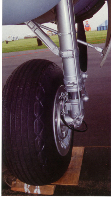
The main gear strut doors were the only open doors when the landing gear was down. A single strut, connected to the main strut assembly, held the door open and closed it during the retraction sequence. (Lou Drendel)
