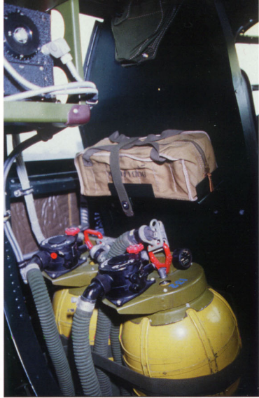
(Above) The area behind the pilot's seats held map and first aid cases, communications and navigation radios and oxygen bottles. Radio and navigation operating controls were on the left and right cockpit sidewalls respectively. Most of the radio and navigation sets themselves were in the navigator/turret gunner compartment behind the cockpit and waist compartment. (EAA photo by Phil High)
