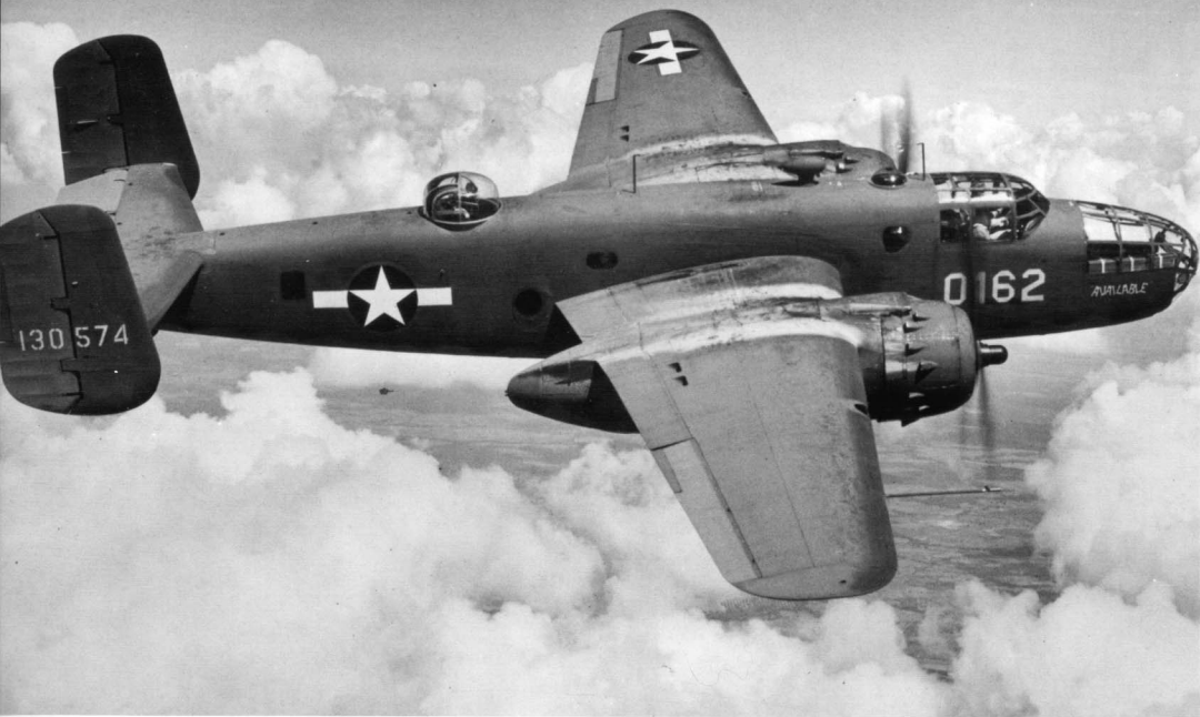
B-25D-20-NC serial number 41-30574 over Kansas in 1942. This is one of 2,290 Mitchells that rolled off the Kansas City production line during WW II. The exhausts have stained and bleached the paint. The paint on the fabric control surfaces has faded at a different rate than that of the painted metal surfaces. (USAF via Norm Taylor Collection.)
