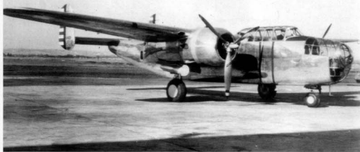
The recently completed NA-40 at Wright Field ready to undergo testing. The NA-40 was a high wing aircraft while the B-25 would be a mid-wing aircraft.
