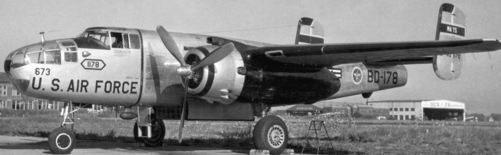
(Above) B-25J-30-NC (44-31178) of MATS, September 1955. The modified exhaust system was common to many post-war B-25s and included a Stromberg carburetor, as evidenced by the higher, narrower intake on top of the nacelle. The new exhaust system collected the exhaust of the top seven stacks and vented it through a single large exhaust port. The windshield wipers are also a post-war addition. (Dave Menard via Norm Taylor Collection.)
