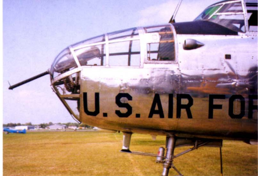
Some wartime aircraft, and many modern restorations, lack the fixed forward firing machine gun. While it carries USAF markings, it is armed like a WW II USAAF airplane (Mitchells were disarmed after the war.) Antennas under the nose are for modern avionics. (Lou Drendel)
