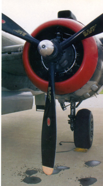
The engine nacelle fully enclosed the main landing gear. This aircraft, a restored B-25J, also has a modified exhaust arrangement. The engine crankcases and reduction gear housing were painted dark gray. The silver ring is part of the ignition system. Oil leaks are also an aircraft's way of life. (Lou Drendel)
