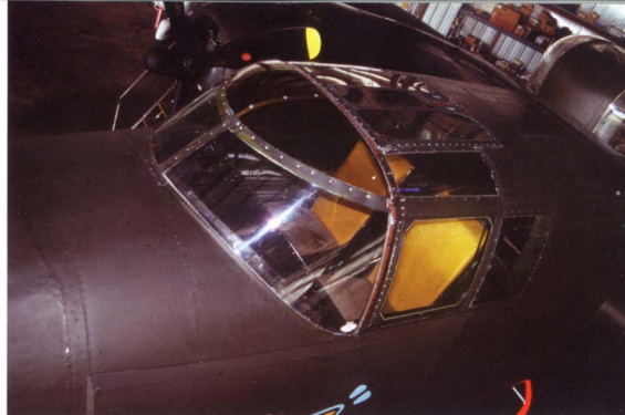
The port side of the canopy. Missing from this restoration is the metal armor panel in the lower half of the pilot's windscreen. (Lou Drendel)
