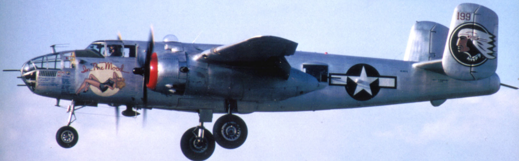
B-25J "In The Mood" on approach to NAF El Centro 11 March 1994. A Plexiglas dome covers the position of the dorsal turret. The B-25H and J had their DF footballs, when fitted, moved to the fuselage underside. (Ted Carlson/Fotodynamics)
