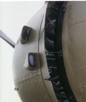
(Right) This exhaust system shows modifications made as a result of problems. The "S" stacks occasionally broke loose from the top cylinder, so a collector ring stack was fitted for the top cylinders, exiting in a single exhaust stack. The lower cylinders retained the original stacks. Cowl fairings were removed and patches installed for the top cylinders, a fairly common modification on post-war B-25s. (Lou Drendel)
