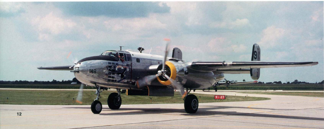
(Below) A B-25J of the Yankee Air Force at Goshen, Indiana 8 August 1996. More highly polished than any warplane would have been, it also lacks a dorsal turret and wartime exhaust system. (Lou Drendel)
