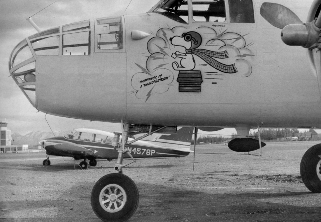
One can only guess at the mission of this civilian B-25J-15-NC, (44-28938) which carried civil registration N7946C at Merrill Field, Anchorage, Alaska, 26 May 1967. The original equipment DF football and wire antennas for the marker beacon (upper wire) and radio compass (lower wire) are still carried under the nose. These have been augmented by at least three modern whip antennas for VHF COM and a larger VOR antenna on top of the nose. (Norm Taylor)
