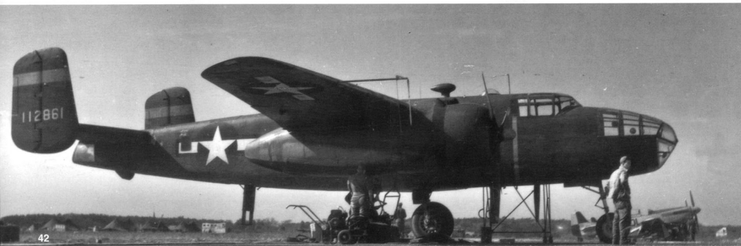
(Above) A B-25C-1-NA (41-13223) of the 377th Bombardment Squadron, 309th Bomb Group, Columbia Army Air Field, South Carolina as it appeared in September 1943. An RDF 'football' antenna is on top of the fuselage. The three fuselage side windows were eliminated on the H/J models. Other significant differences visible in this view include a smooth engine cowl and no tail gunner position. (Norm Taylor Collection.)
