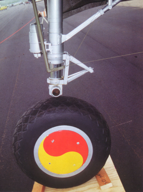
B-25s employed tricycle landing gear. The nose gear, known as the auxiliary gear in USAAF parlance, was equipped with a 30 inch, 8 ply tire. The nose gear was not steerable but could caster up to 60 degrees left or right. The spoked wheels were often covered with a plate. (Lou Drendel)
