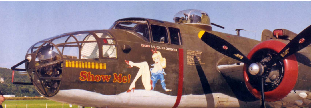
B-25J "Show Me!", flown by the Missouri Wing of the Confederate Air Force, is equipped with two fixed forward-firing machine guns. (Lou Drendel)
