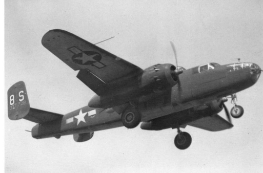
B-25J-1-NC (43-27729), assigned to the 488th Bomb Squadron/340th Bomb Group/12th Air Force, landing at an American base on Corsica in March 1944. This was among the first production J models and lacks the factory installed fuselage gun packages. (Norm Taylor Collection.)
