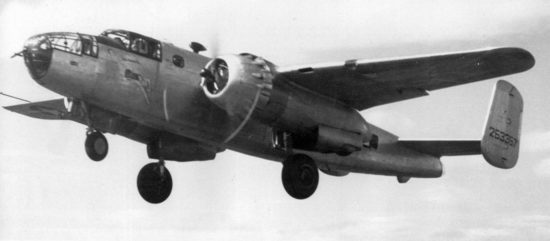
The transitional position of the landing gear doors is visible as this B-25C-5-NA of the 7th Photo Group departs from Mt. Farm Airfield, England in the spring of 1945. The landing gear retracted aft in about 16 seconds and extended in about 10 seconds. The main and nose wheel doors opened only during the retraction or extension sequence. (Robert Astrella via Norm Taylor Collection.)
