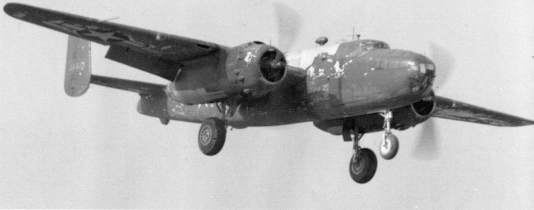
A very well-worn B-25C of the 12th Bomb Group landing in Italy during W.W.II. The use of unimproved forward airfields, with flying dirt and stones played havoc with propellers and paint in combat conditions. Under such conditions, having the main and nose gear doors closed to keep out debris was probably a good idea. (Norm Taylor Collection.)
