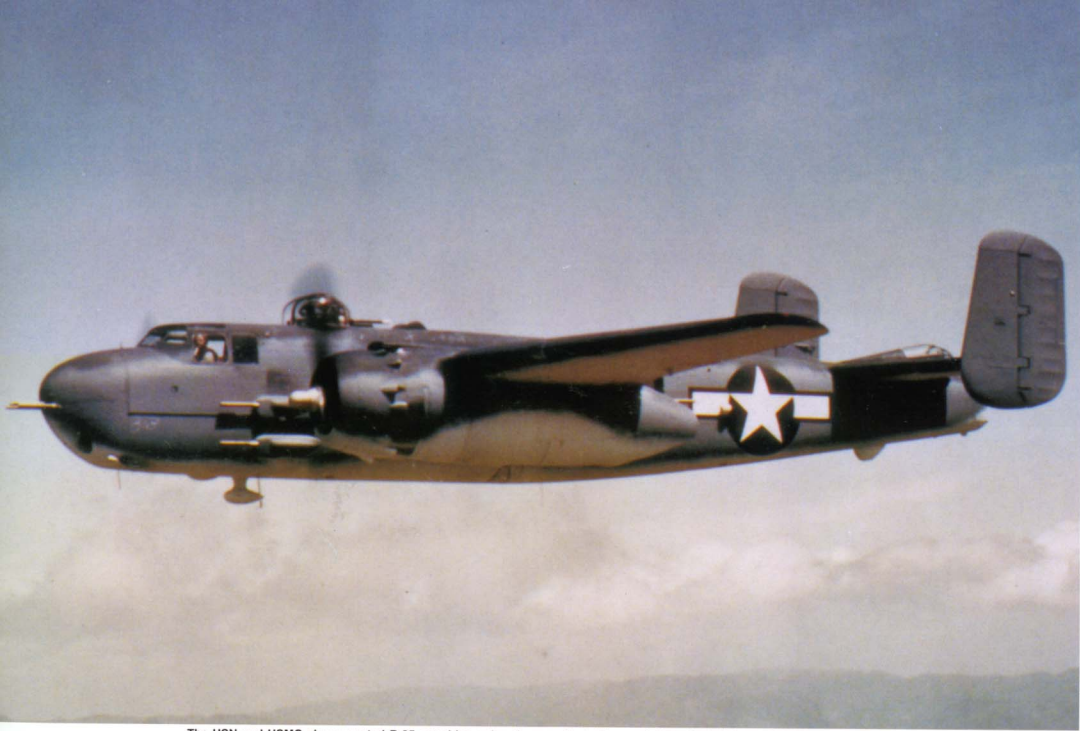
The USN and USMC also operated B-25 gunships using them against ships and shore installations. With the exception of some minor details, they were fairly similar to their U.S. Army counterparts and used the same weapons packages. Some late Marine B-25Gs also had a manned tail gun position with an overhead canopy. Due to their extensive over-water missions, the Navy and Marine's B-25Gs and Hs were camouflaged in the tri-color scheme of Sea Blue, Intermediate Sea Blue and White. In naval parlance, B-25s were known as PBJ-1s.
