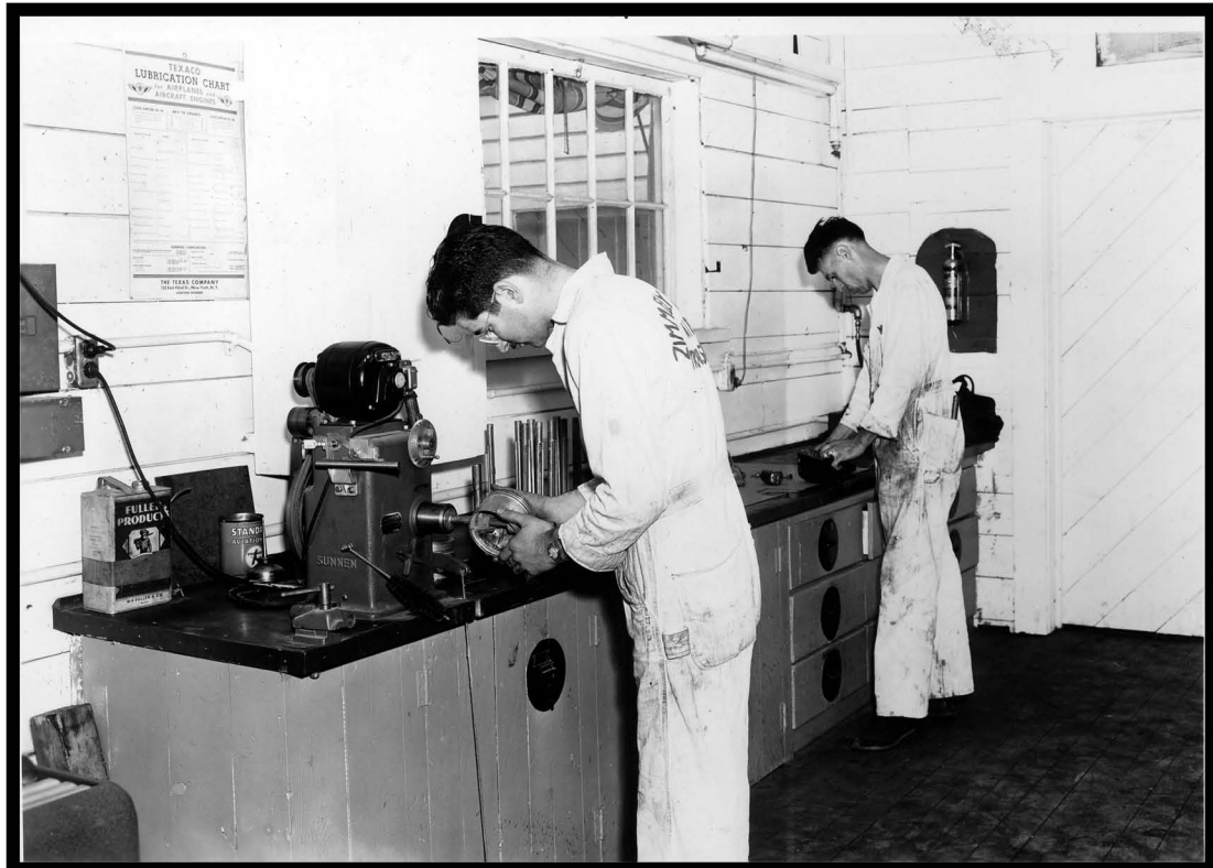
Lower Picture No. 21. Frank Brockway, operating the Sunnen Reamer. Earl Clark, overhauling a carburetor. We have all parts and complete testing equipment for carburetors.
