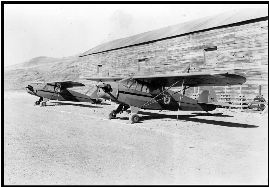
Below: Two trainers illustrating the tie-downs used for all training planes. These tie-downs conforming to WTS specifications assure adequate protection from strong winds which may occur while planes are not hangared.
