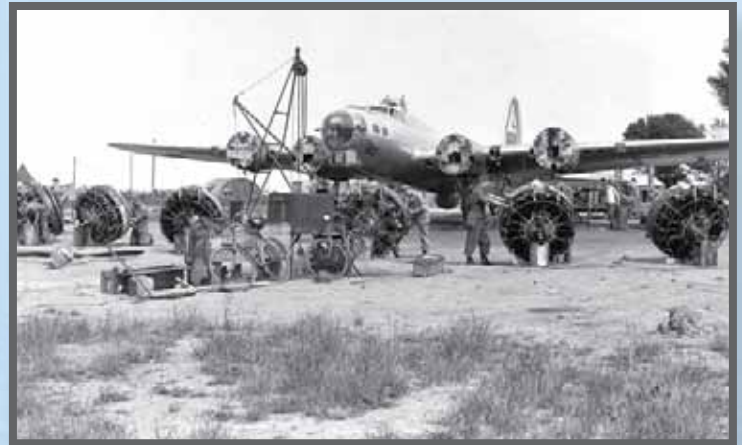
An engine change for B-17 hit by German fighters on a mission over Berlin.
