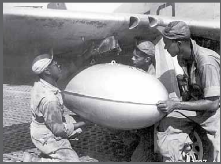
Tuskegee Airmen ground crew members load a wing tank on a P-51 Mustang.
