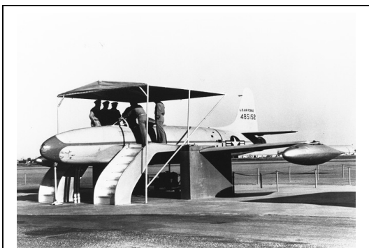
The Captivair “synthetic” trainer, which simulated flight conditions in the T-33. (USAF Photo)
