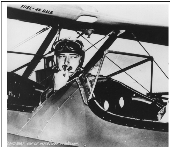
Instructor, with the mouthpiece, and student, with earphones only, using a Gosport system. (USAF Photo)
