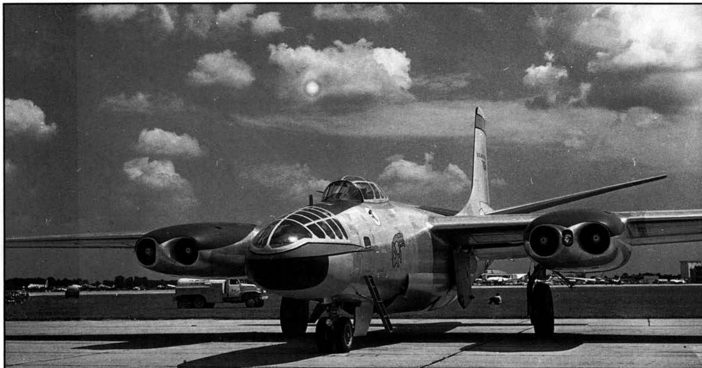
The B-45 had excellent crew accommodation. Its main drawback was the restriction of forward vision for the co-pilot by the front pilot's ejection seat, due to the tandem arrangement. Crew of four was carried, including a gunner in the tail compartment armed with two .50cal machine guns.
