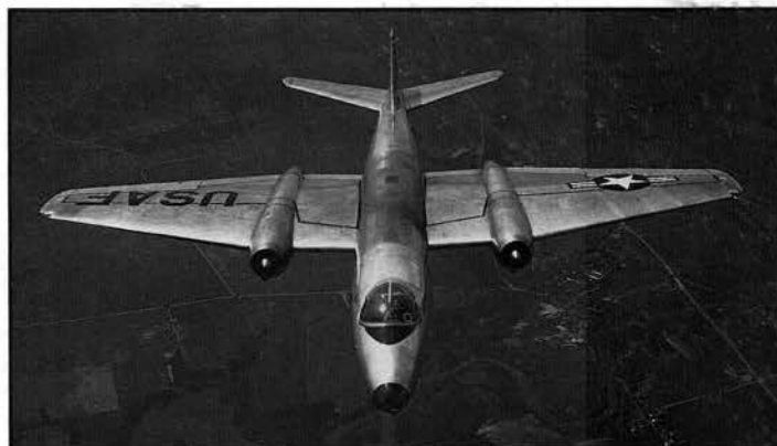
This is the American Martin-built B-57 which was developed from the British Canberra. There is no noticeable exterior differences. The interior layout of the British Canberra was three place with two crewmen seated side by side behind the pilot. The American B-57 had only two crew positions, the second being seated low and behind the pilot. (Martin)
