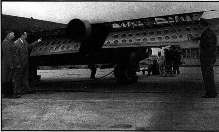
Four landing flaps provided considerable surface area. These were two-position hydraulically operated and air-load balanced.
