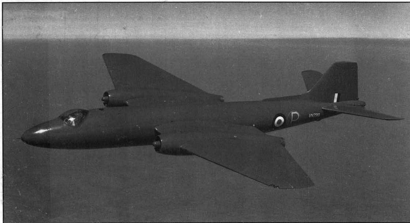
The Avon RA2 powered prototype Canberra in the air. Tip of rudder has already been trimmed which proved necessary after the first flight. Dorsal fin was eliminated on production models. Bareheaded Beamont can be seen in the cockpit of the blue painted craft. (BAC)
