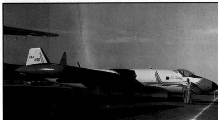
The FAA acquired two RB-57As for use in flight testing the high altitude jet route structure. N96 was formerly 52-1438, while N97 was 52-1447. This FAA Canberra N96 crashed in 1960 when the pilot had to eject when the control column inadvertently disengaged as part of the emergency ejection system.
