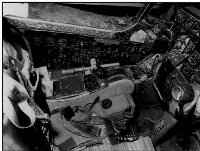
Most noticeable change over the years for the B-57 cockpit was the introduction of the Douglas ESAPAC rocket ejection seat. It could take the seat high enough for ground level escape provided there is sufficient forward speed for chute deployment. A heavy blade knife designed for the nearly impossible task of cutting through the canopy was on a holder below the windscreen.
