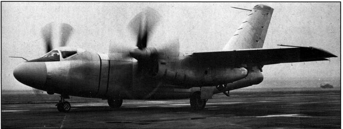
North American offered an alternative to the AJ-1 Savage, the A2J-1 featuring turbo-props and other refinements. Its development could incorporate the Air Force requirements, but the prospect was shelved in lieu of more advanced designs. (North American)
