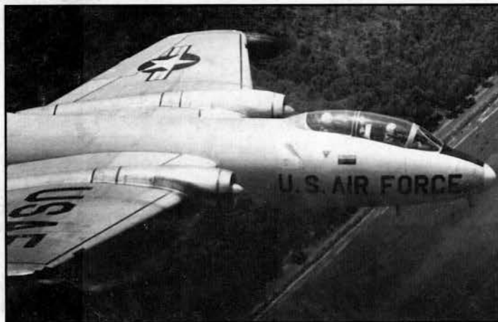
The B-57 proved to be the best airplane in SEA for night intruder missions the purpose for which it was selected 14 years before. Good visibility from the cockpit without structural hindrances was a marked feature. It could be slowed in flight sufficiently for the crew to have time to pick out targets and line-up on an attack run. Good loiter time and large bomb loads were also important assets.
