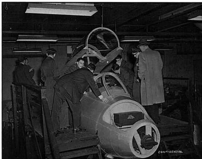
Mock-up of Martin's redesigned nose section is evaluated closely by Wright Air Development personnel. This model became known as the B-57B, its cockpit reflecting American styling throughout. This redesign was necessary in order to provide a windshield with flat glass behind which to place a gunsight without having distortion due to temperature and pressure changes. (Martin)
