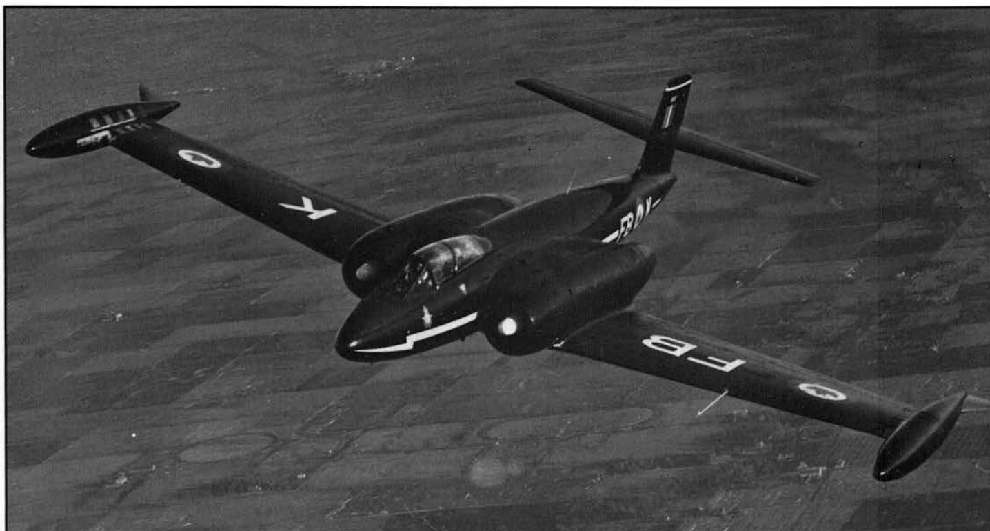
The CF-100 built by A. V. Roe Canada Ltd was a very new fighter nearing production status. It was soon learned that it did not have the potential for being a jet bomber, yet those who flew it gained much in evaluating the all-weather and night flying qualities that could be built into such an aircraft.
