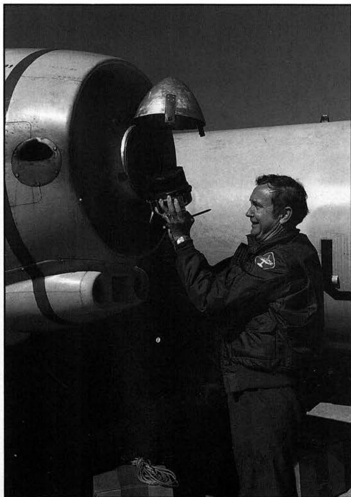
The author removes the expended starter cartridge at the end of the delivery flight of 551 to the National Air and Space Museum. These cartridges were for a one time start and dependent upon good electrical contact points despite the dirt from the burning material that this system emitted.
