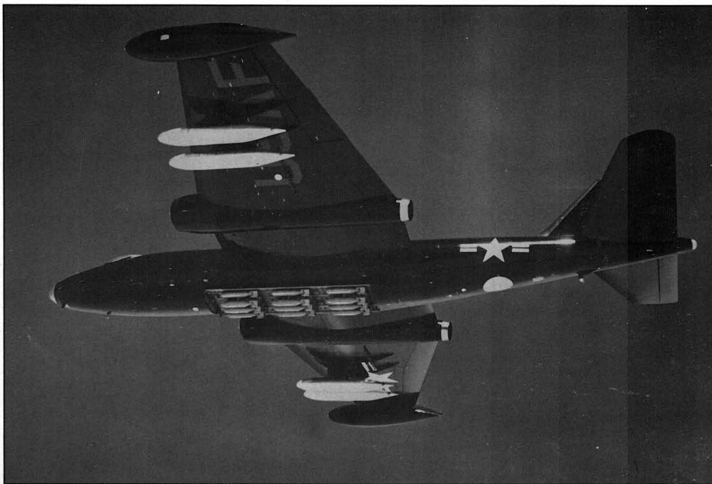
Externally, the Martin built RB-57A showed no structural design changes to that of the British Canberra. The Martin-built Canberra contained their in-house devised rotating bomb bay door that eliminated buffeting when opened at high speeds over that of the clam-shell door type. Photo-flash bombs are shown attached to the door. (Martin)
