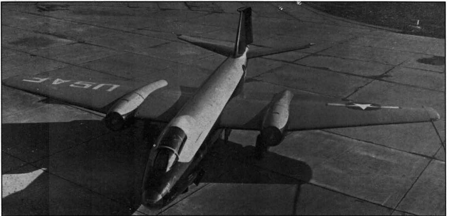
Former Canberra WD940 was modified by Martin with this new tandem canopy for engineering study and was possibly used for flight evaluation. This led to the B-57B. The clear forward nose section was left unchanged for this evaluation. This elongated canopy adds even slimmer lines to the Canberra. (Martin)
