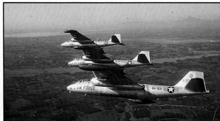
Three B-57s of the 3rd BW in Japan make a formation turn above the Kanto Plains. When the 3rd assumed the nuclear strike mission in the Far East, their 70-83lbs of black paint that had not held up well in the first place, gave way to unpainted, more heat reflective natural metal skin.
