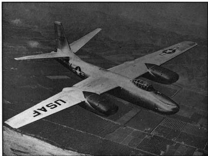
North American B-45 Tornado had promise in the night intruder role, but its structure was based upon World War II design. Two engine nacelles housed its four jet engines. With four engines it had good partial engine performance. Pilots rated it easy to fly.
