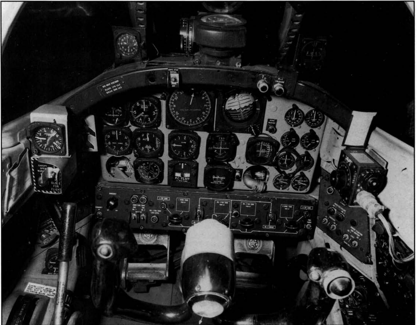
Instrument panel of the B-57 was conveniently arranged. Flight instruments were grouped at center and left, and engine gauges were at right. Fuel control panel was laid out in schematic format, with engine fuel shut-off wafer switches already converted to toggle switches but not shown safety-wired to 'on' position in this picture. Stabilizer trim indicator above canopy switch at left. (D. Beggerly)
