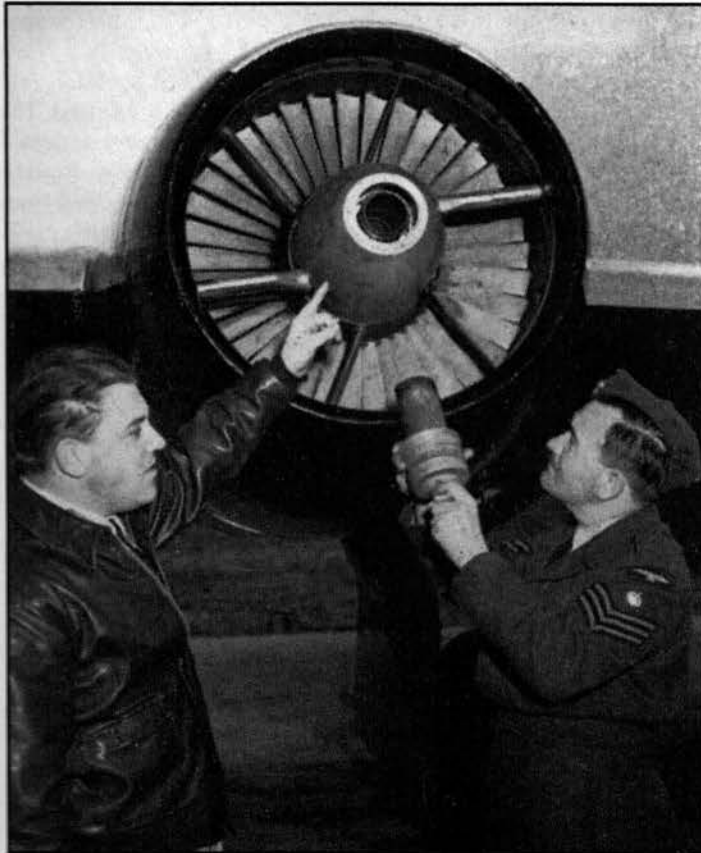
The Rolls-Royce Avons on this early model of the Canberra were started by a powder-charge cartridge positioned in the nose of the engine. Later Canberra models carried three cartridges, while the Americans when using the Sapphire retained the single shot starter charge but of a larger size.
