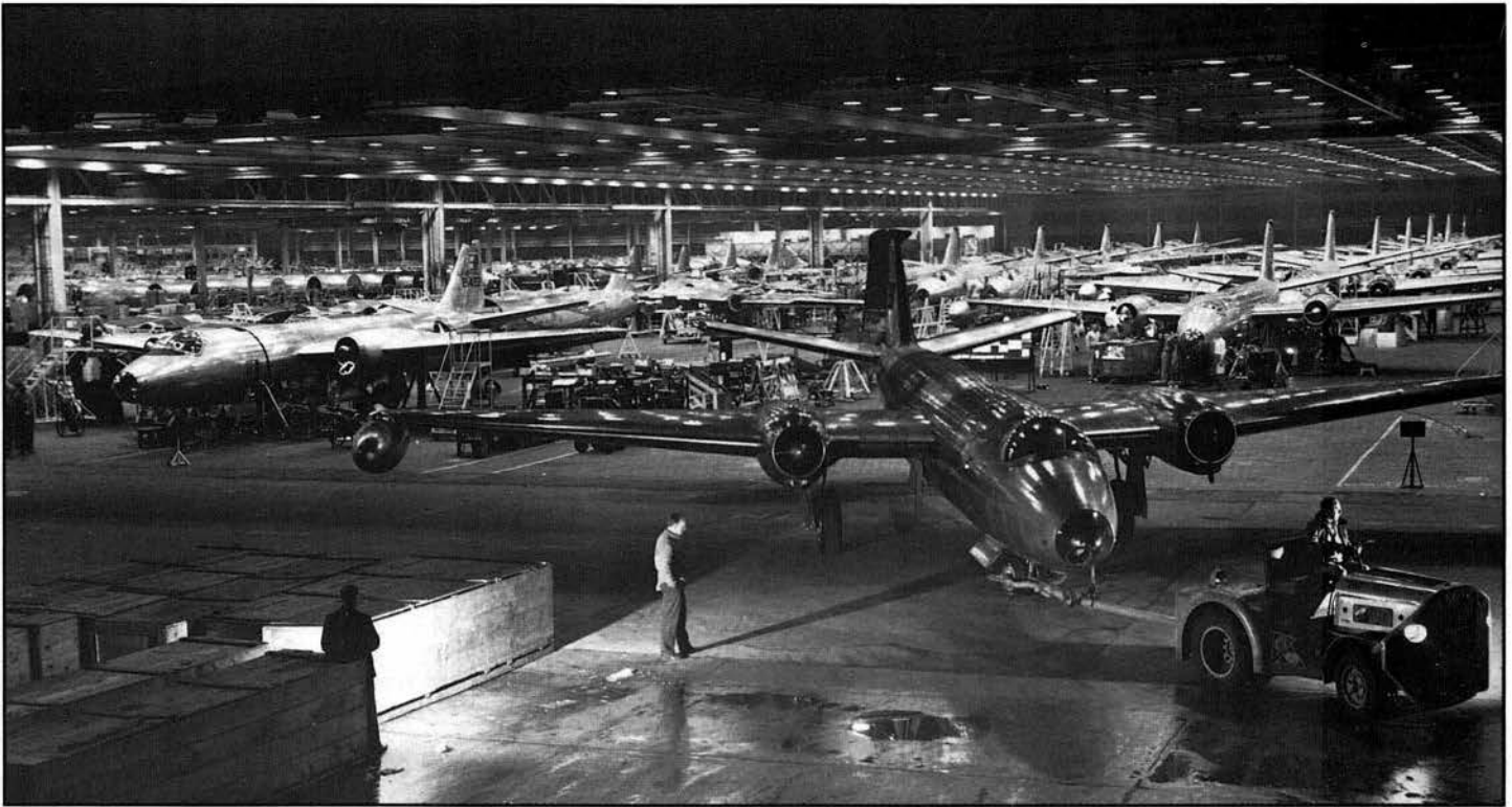
The setting sun did not halt production of the B-57, spurred on by the war in Korea. Two work shifts were employed by Martin, until the first four bomb groups were outfitted. RB-57A in foreground is being towed to the paint shop for its coating of anti-searchlight black paint, while B-57A, ship No 5 (52-1422) at left, already has its markings and was left in natural finish. (Martin)
