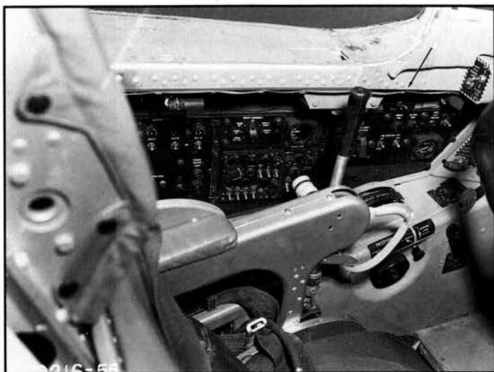
This original B-57B cockpit configuration shows dive brake toggle switch under canopy ledge (arrowed), and stabilizer trim gauge on lower right side panel. Emergency hydraulic hand pump handle was normally stowed. This thruster type ejection seat was replaced in early 1970s. (USAF)
