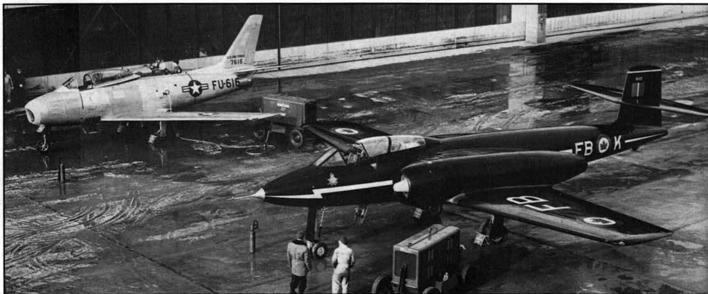
The CF-100 was most unusual in design with its thick center section joining the two 6,000lb thrust Avro Orenda turbojet engines. With addition of tail warning devices to detect attacks at night or in weather, the evaluation committee graded the CF-100 able to survive combat encounters well beyond its anticipated operational life span. One measuring yardstick was ability to defend against attack by F-86 type fighters as seen in the background. (Avro)
