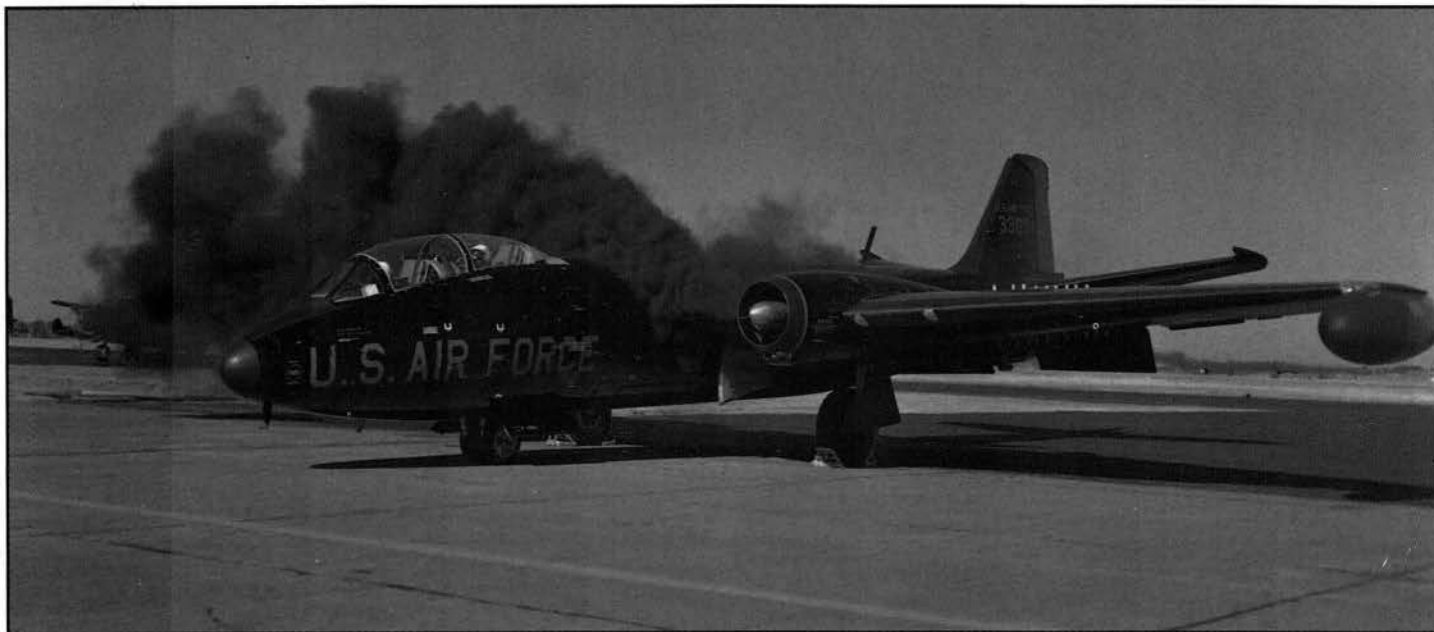
The engine start of a B-57 was immediately obvious by 10 seconds of black smoke that belched from the starter exhaust of each engine. The right engine was started first to build-up hydraulic pressure so that the canopy could be closed to protect the crew from the left engine starter smoke. Clean burning starter cartridges were later developed. (USAF)
