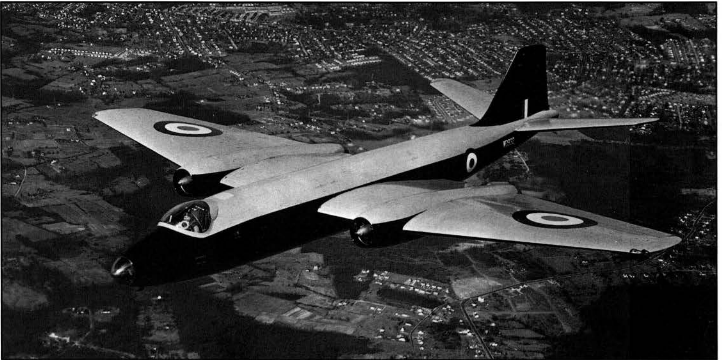
Early English Electric Canberras like this B Mk 2 were powered by Rolls-Royce Avon 101 engines of 6,500lb thrust as compared to the J65 Sapphire with 7,200lb of thrust built under license from Armstrong Siddeley which powered the Martin B-57. The Canberra design was void of defensive armament, relying on its speed and maneuverability to escape interception. Martin's B-57 was developed from this variant.
