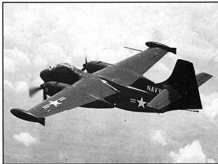
Another North American product in the evaluation was the AJ-1 Savage. This was already in fleet service but showed little growth potential for the Air Force requirement. Augmenting two R-2800 radial engines was one J33 turbojet buried in the aft fuselage area. (North American)
