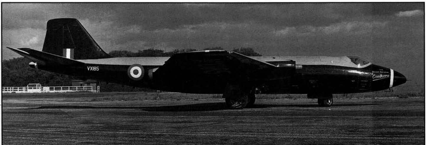
Since the Canberra was one of the very early jets of this relatively large size, its low stance with the ground seemed most unusual since propeller clearance was no longer a problem. This gave great ease to ground maintenance of the engines and other accessories. Cockpit entrance was one long step up to floor level through the nose hatch under the canopy. (BAC)
