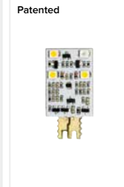
# 4941C Bayonet mounted LED (3 white LED'S + 1 red LED)
