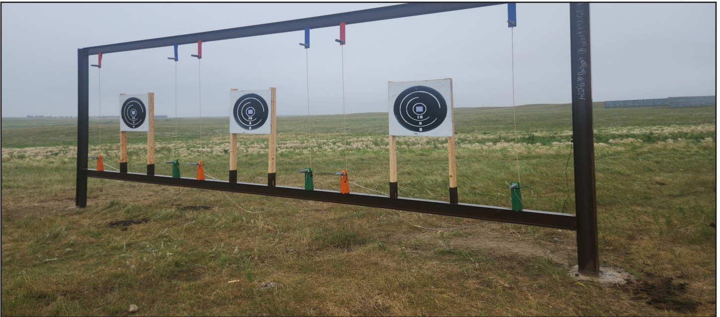
Target frame with aiming points and Shotmarker sensors attached.
