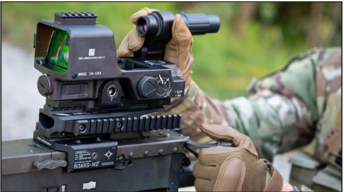
Type classified as the M155 Mounted Machine Gun Optic, or MMO, the sight attaches to the M2A1 .50 cal with a BE Meyers BOARS Mount using M1913 Picatinny rails. (Photo: U.S. Army Capability Program Executive -
