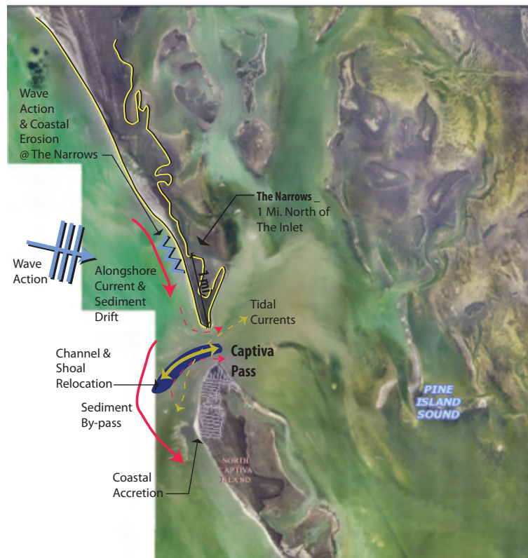
The Captiva Pass Inlet System _ A Complex Coastal Inlet System w./The 480-ft. +/- Wide Management Zones CC-10A & CC-10B Corresponding To The Narrows , An Area Noted For Dynamic Coastal Change Approx. 1 mi. North Of Captiva Pass
